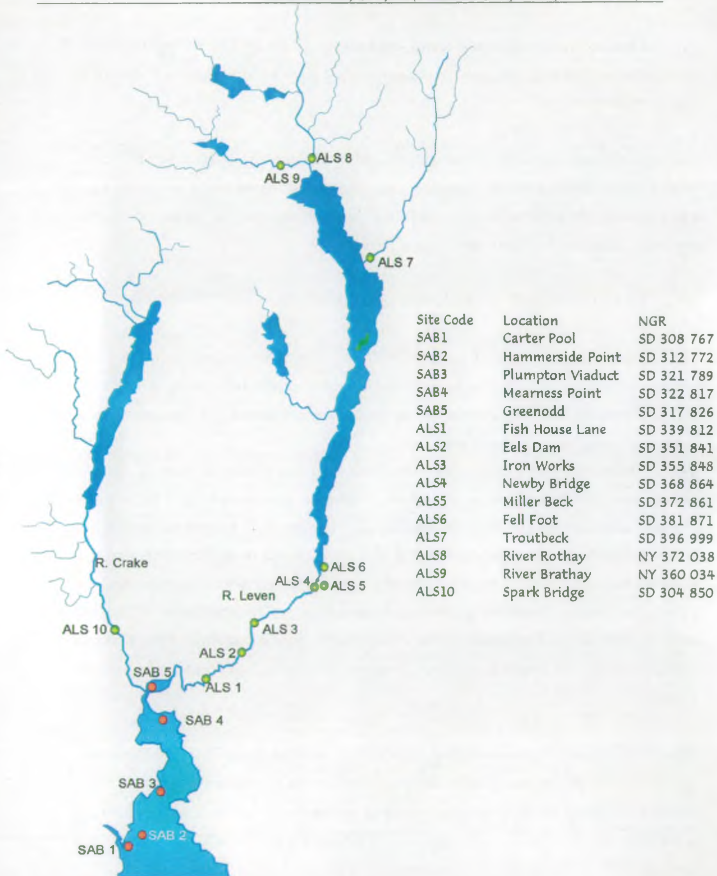
Figure 3. The Leven estuary with Leven and Crake catchments showing sonar buoy and listening station locations.
