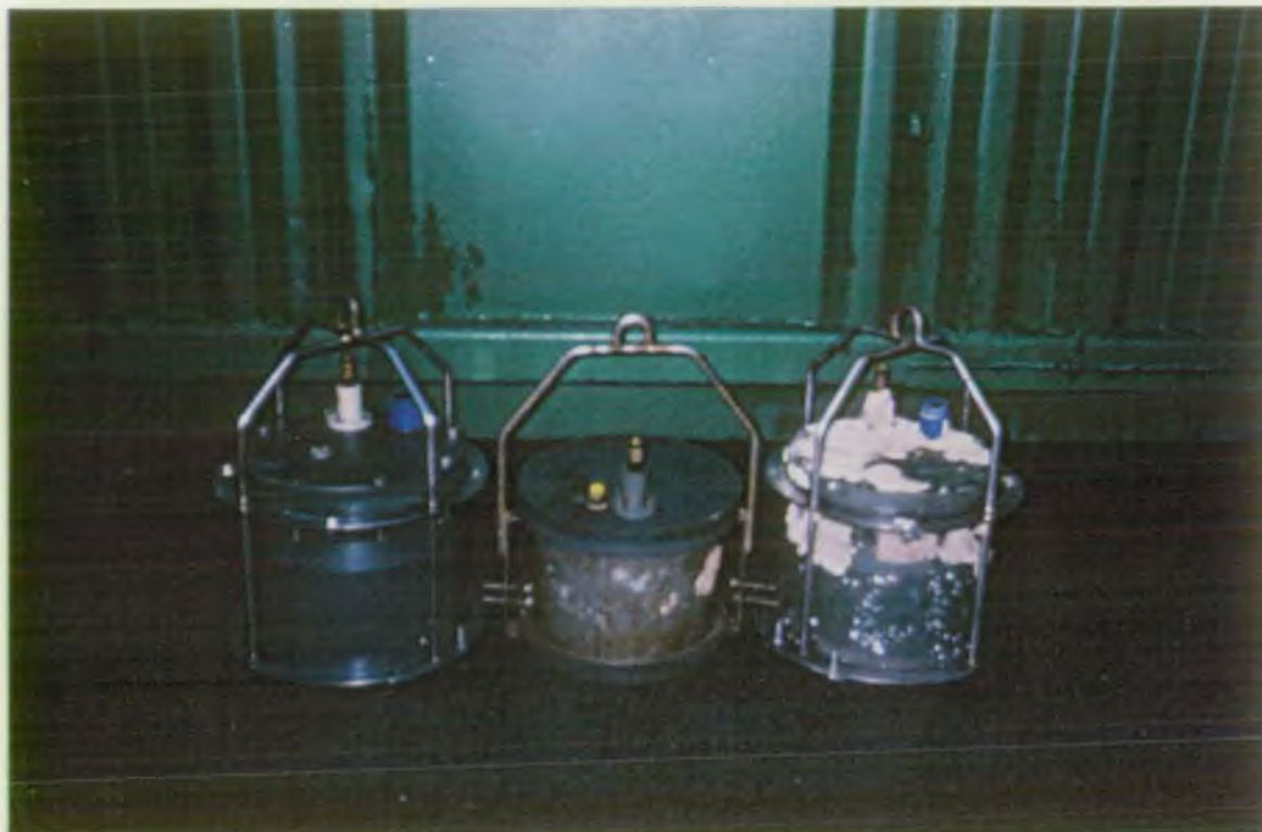
Plate 1. Sonar Buoys (Hammerside Point buoy far left) illustrating barnacle growth.
