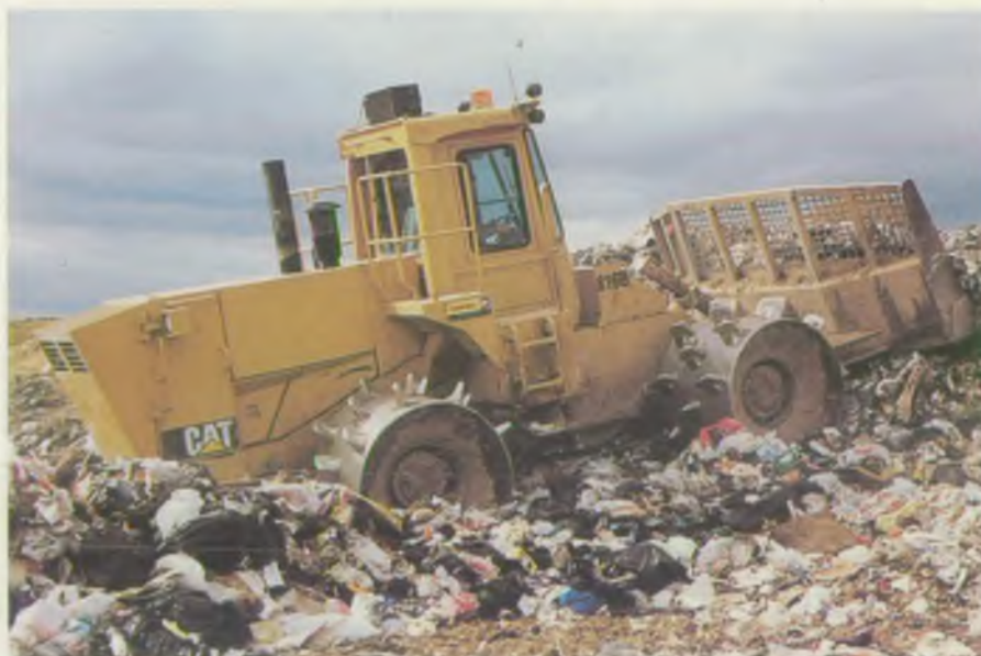
Compacting waste at a landfill site
