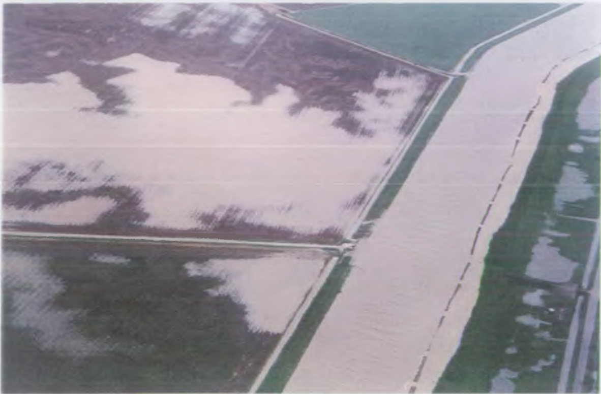
Figure. 8e: Overtopping Of The Cradge Bank At Bell Row Freshwater Feed, 11/04/98
