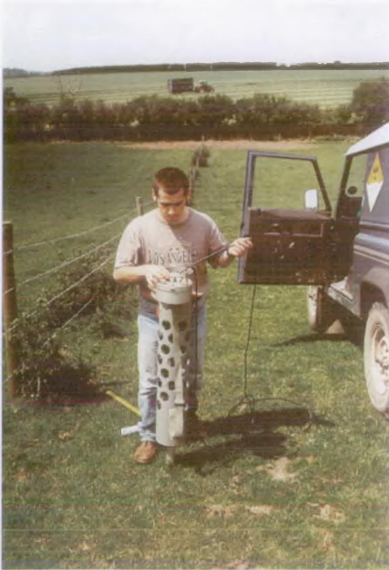
**Plate 3 Measuring soil water content in the Pang catchment using a neutron probe**
