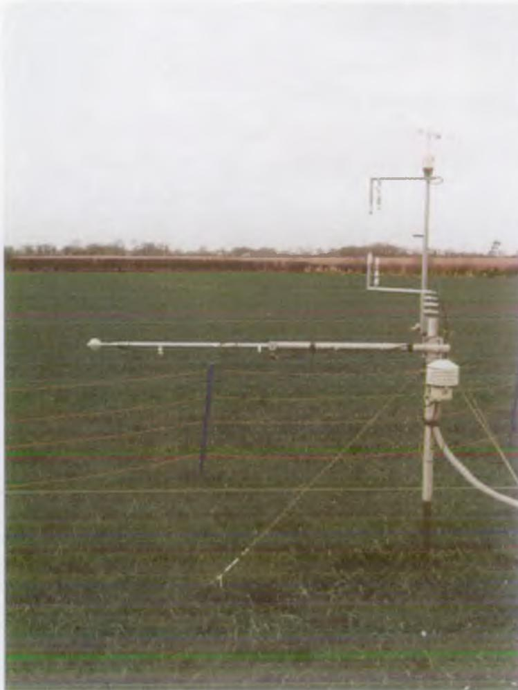
**Plate 1 The IH Hydra sited adjacent to the Bacon Hall soil moisture monitoring site in the Tern catchment**
