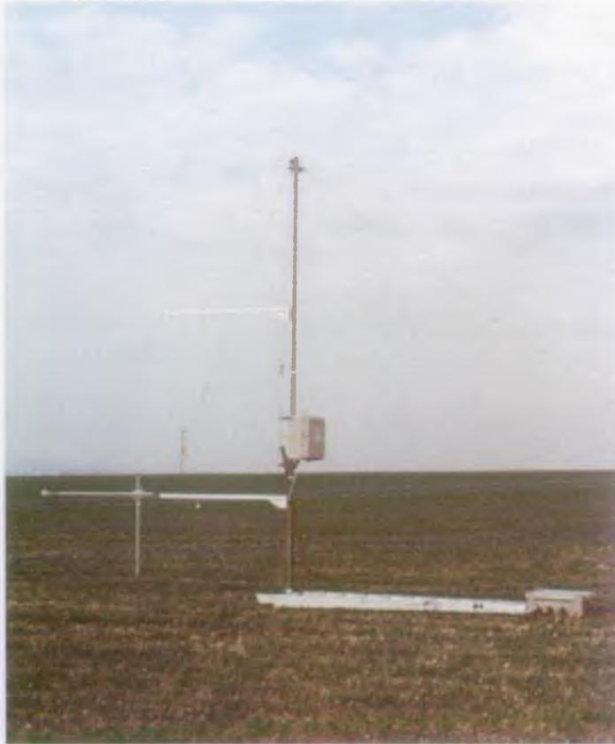
**Plate 2 The Bowen ratio machine at the soil moisture monitoring site 10 in the Pang catchment**
