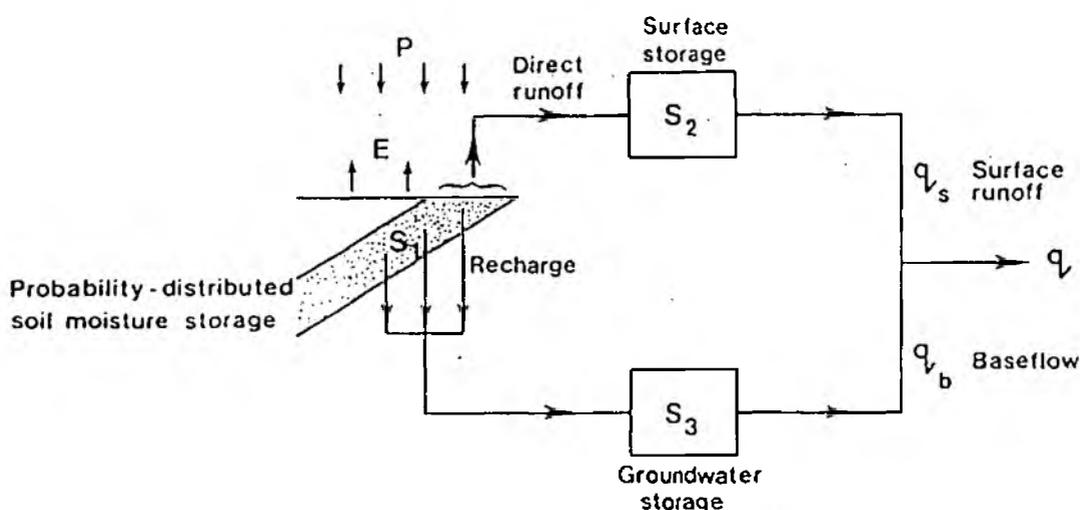
Figure 3.4.1 The PDM rainfall-runoff model
