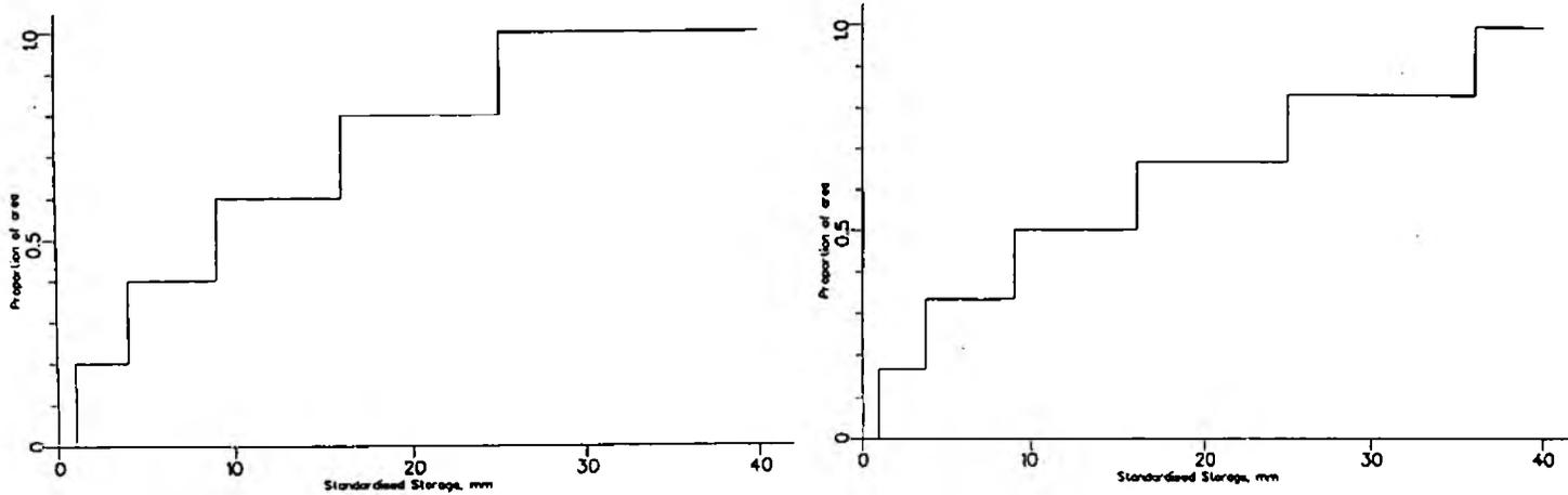
Figure 3.5.2 Runoff production component of the SUHM model: distribution functions of storage capacity, in standardised form, used for paved and riparian areas
