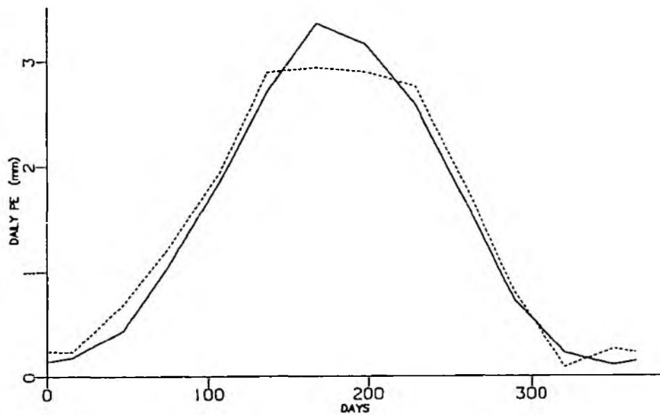
Figure 2.5.1 Daily potential evaporation profile in mm for the standard year (solid line) and for 1988 (dashed line) for the Upper Mole
