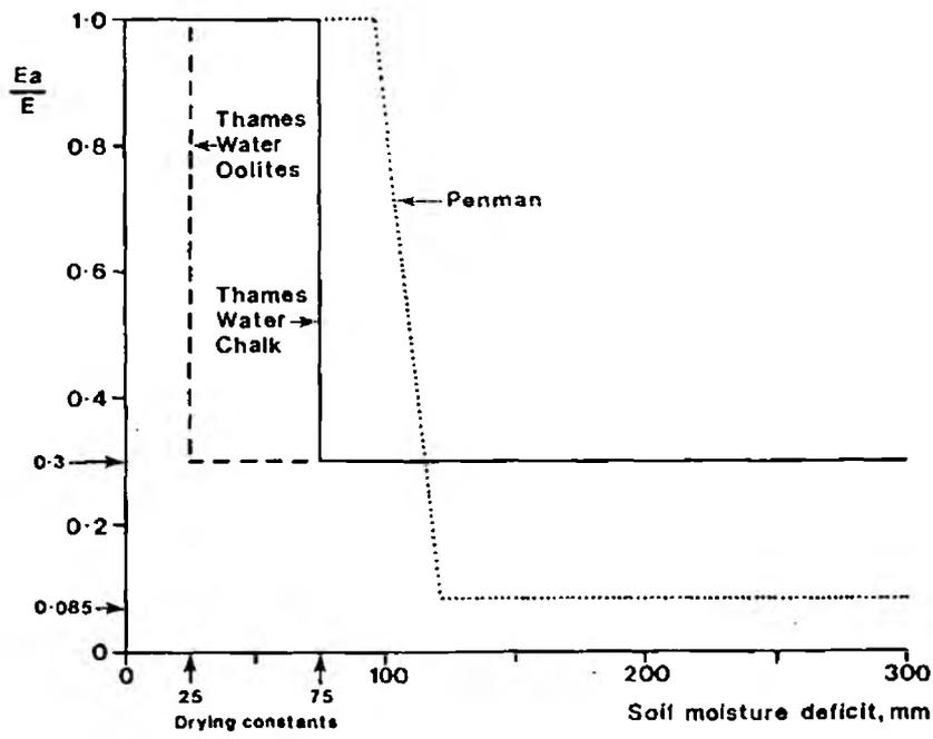
Figure 3.2.2 Representation of actual evaporation,  $E_a$ , as a function of potential evaporation,  $E$ , and soil moisture deficit
