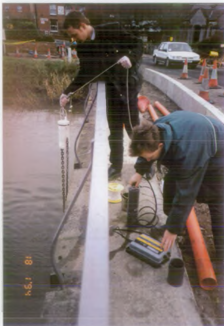
8.1 Use of Casella Sampler (left) and Grant/YSI Logger (Right) at Burrow Bridge
