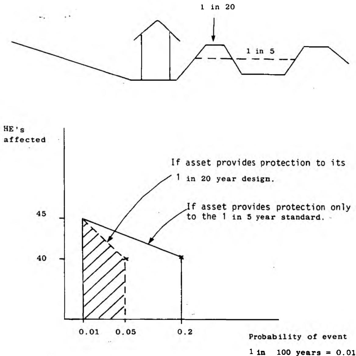
The area under the graph equals the HE's likely to be affected per year by flooding. This must be expressed on a per km basis to allow comparison. Assume reach length = 4km.
