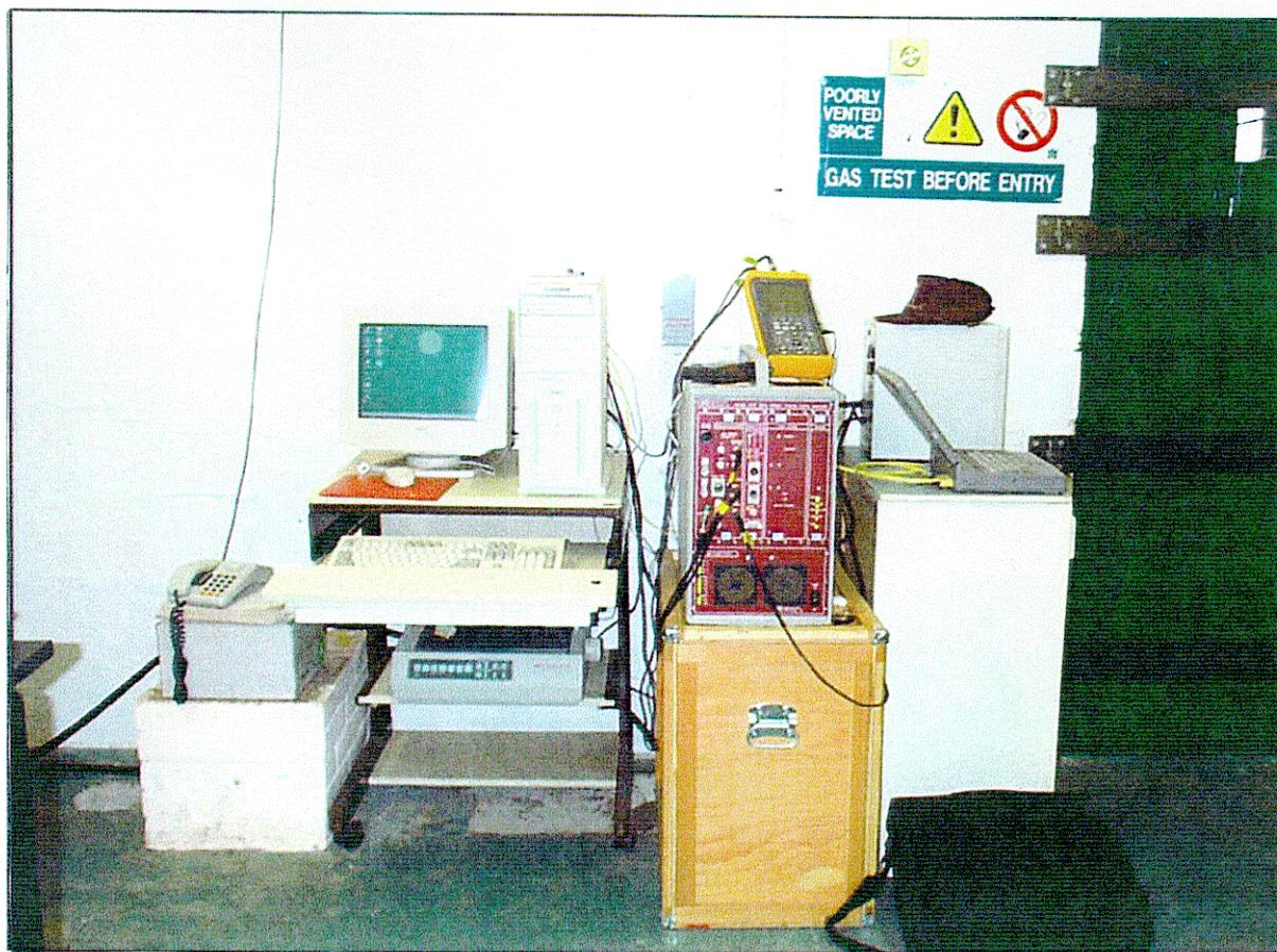
Figure 4.1. HTI echosounder, echo processor and peripheral equipment deployed on site.
