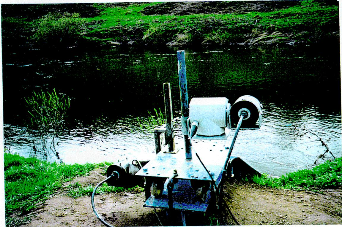
The transducer is attached to a trolley that can be winched down a slide. In this picture, two transducer/rotator pairs are mounted on the trolley.
