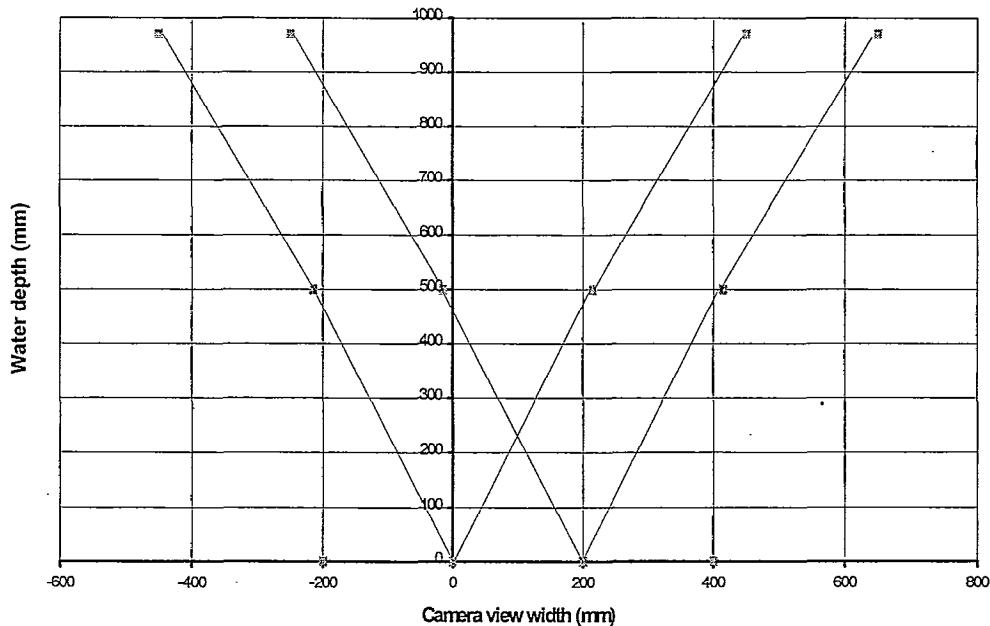
Figure 5.22: Video camera field of view.
