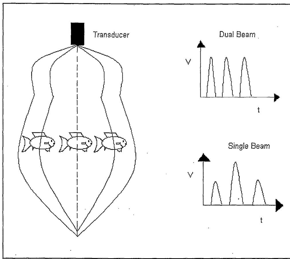
Figure 2.1. The output voltages from an echosounder due to fish swimming through a dual-beam and single-beam acoustic beam.
