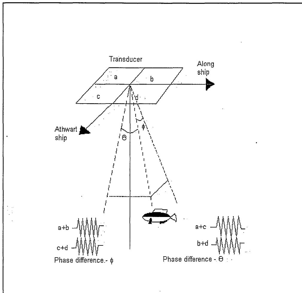
Figure 2.2 Diagram showing the principles of a split-beam echosounder from the perspective of a vertically aimed transducer.
