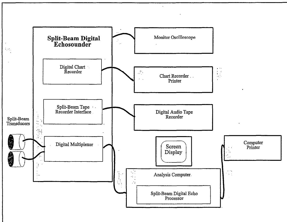
Figure 4.2 Diagram of the Model 243 Split Beam system used on the Wye
