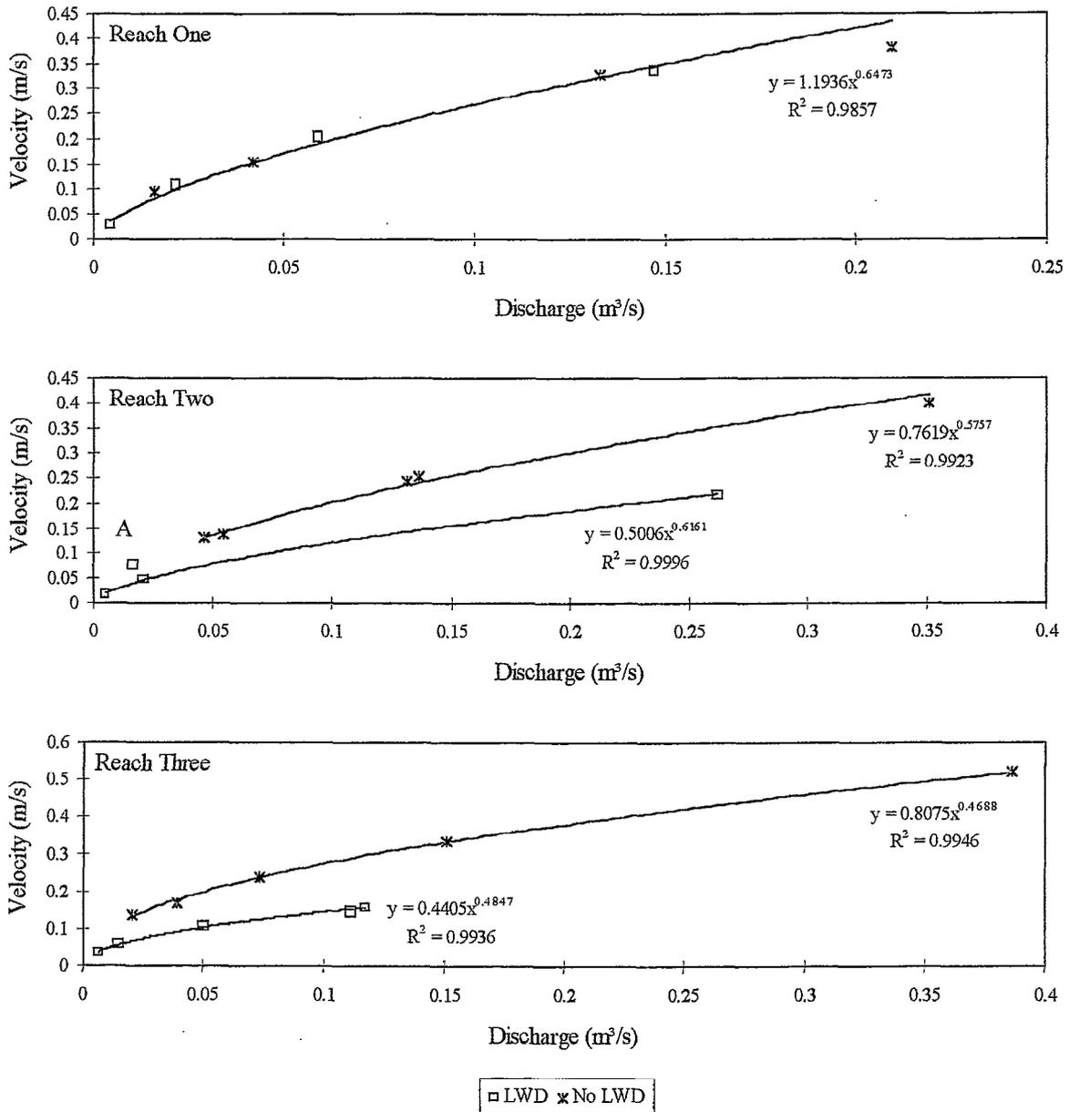
**Figure 3.2 Reach mean velocity for Forest of Dean experimental reaches with and without LWD.**
