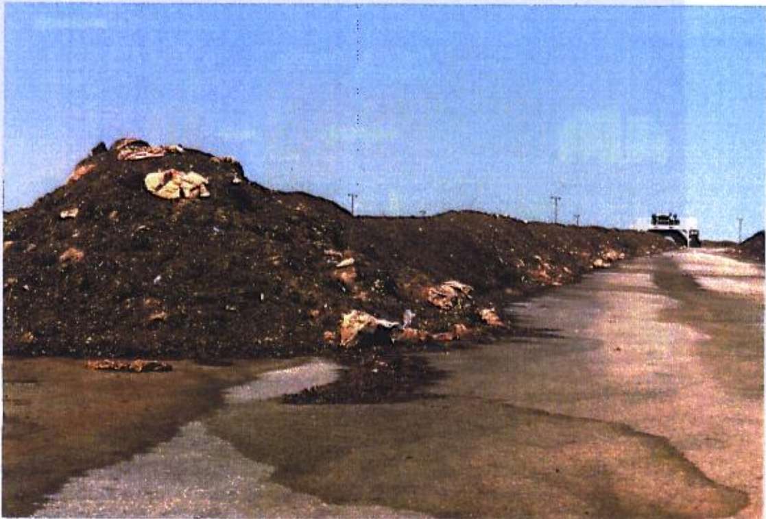
Figure A1.5: Composting Operation Showing Windrows
