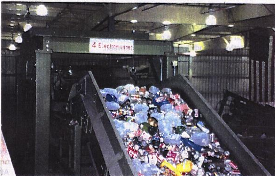
Figure A1.2: Electromagnetic Separation of Ferrous Metals in a MRF
