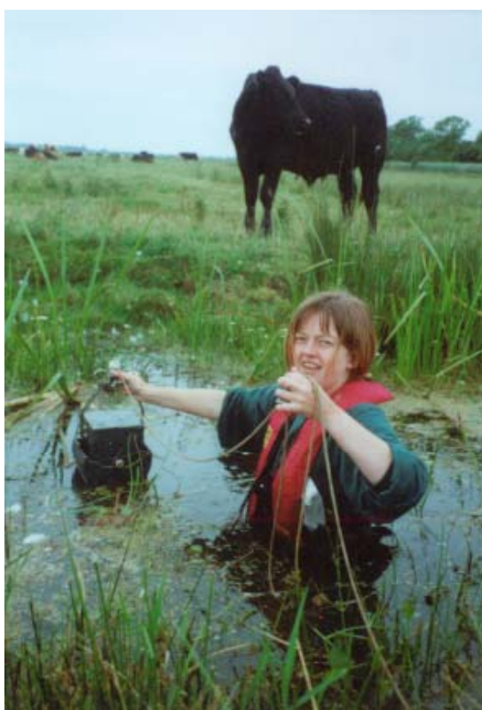
Above left: Using an Eckman grab on a rope, it was decided to use a pole-mounted Eckmand grab which provided greater control of collection. Above right: The GRANT 3800 meter was used to record pH, conductivity and dissolved oxygen in situ.
