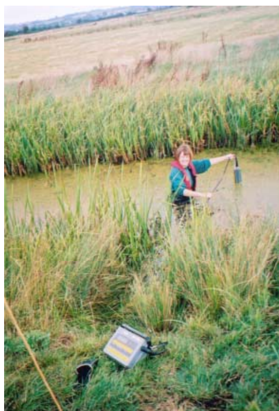
Above left: Using an Eckman grab on a rope, it was decided to use a pole-mounted Eckmand grab which provided greater control of collection. Above right: The GRANT 3800 meter was used to record pH, conductivity and dissolved oxygen in situ.
