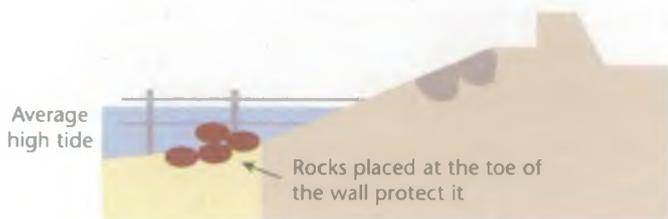
Figure 4 Use a rock toe to protect the wall, option 4
