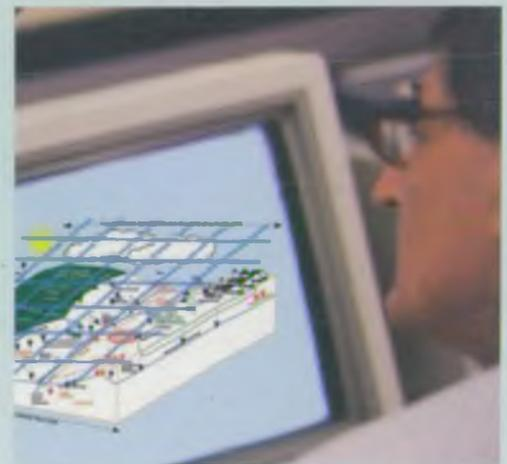
**Stage 3** is to develop a grid-based computer model (termed a Distributed Groundwater Model) capable of representing flows within the project area. The model allows the interaction between rainfall, groundwater, surface water (rivers, lakes etc) abstractions and discharges to be quantified. The impact of changes to the existing regime e.g. from the licensing of a new groundwater abstraction borehole, can therefore be quantified.
