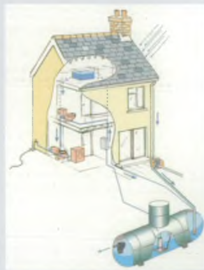
Rainwater recycling: designs like these can make water savings of up to 25 per cent
