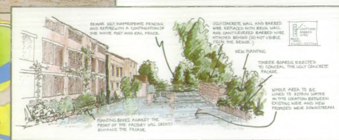
The ugly concrete edge would look far more attractive if faced with timber boards (below).
