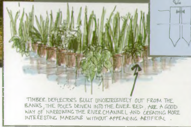
Timber deflectors can be used to mimic natural rafts of vegetation (left). Poles driven into the river bed can create spits of vegetation that can also form a narrowing of the channel.
