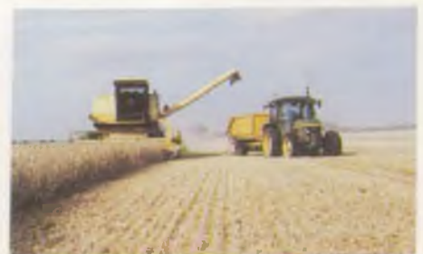
Combine Harvester: many use a closed radioactive source for crop flow measurement.
