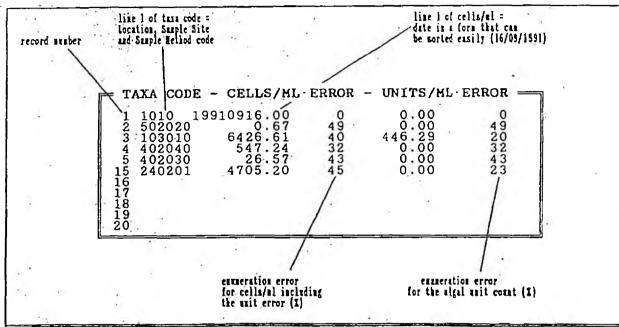
FIGURE 11. 1 Layout of basic data base, showing 20 records. Line 1 holds the location, sample site and sample method code, followed by the data in a form which allows rapid numerical sorting. Unit error is the enumeration error for the units/ml count, whereas the cells/ml error is the cells/unit error combined with the unit enumeration error (where applicable). Lines 16 - 20 are empty.
