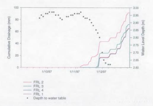
Figure 8.15 Soil drainage predicted by FRL and observed water levels at Stoke Bridge
