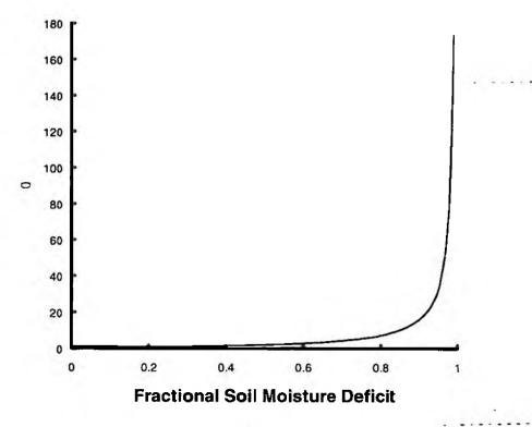
Figure 7.1 The MORECS model of surface resistance as a function of soil moisture deficit
