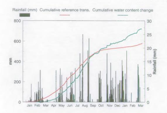
Figure 6.13 Reference transpiration and changes in soil water content at tube 7
