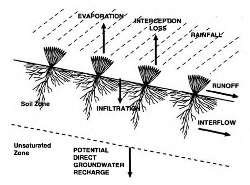
Figure 2.1 Schematic representation of the water balance
