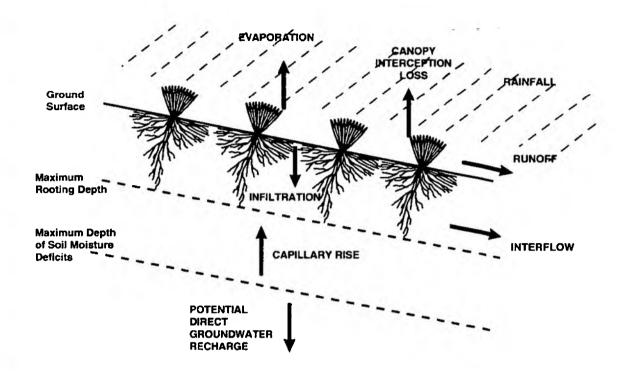
Figure 10.1 Schematic diagram of the conceptual model of direct groundwater recharge
