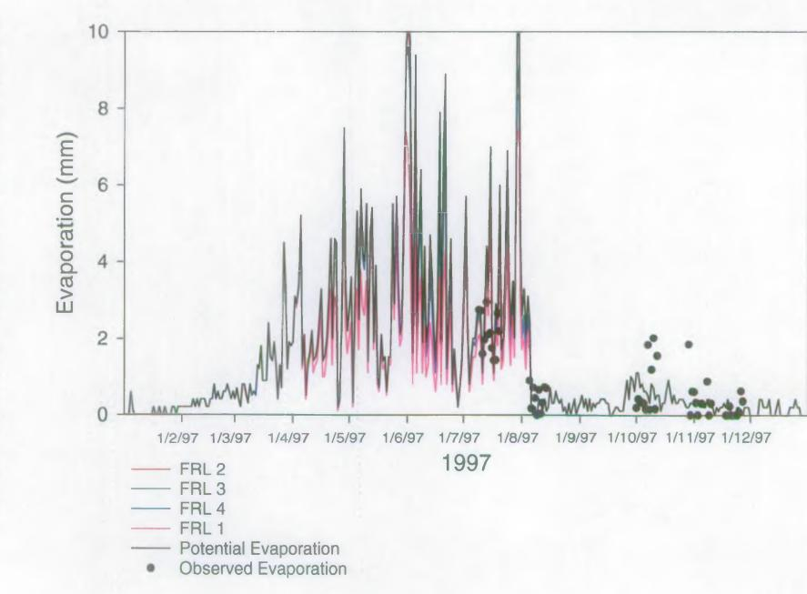
Figure 17.1 Observed evaporation and that predicted by FRL at Site 10
