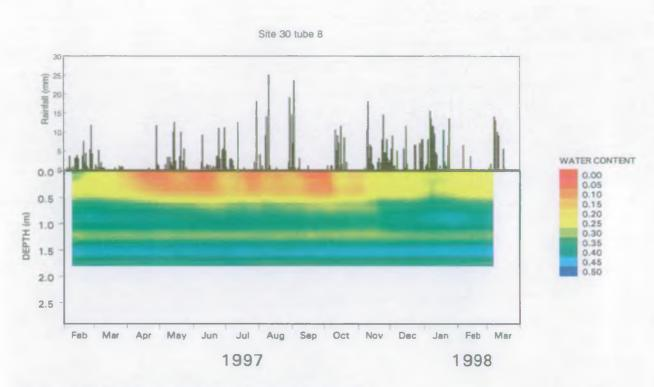
Figure 6.5 Changes in soil water content at tube 8
