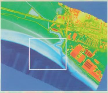
Detailed height measurements in the Humber Estuary from LIDAR
