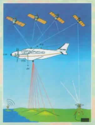
LIDAR system: Operational links
