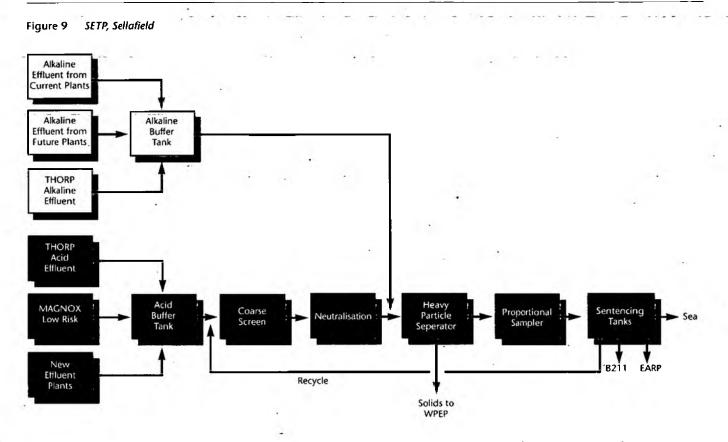
As levels of radioactive caesium in the waste feed are relatively high, removal of this is assisted by addition of pre-prepared nickel hexacyanoferrate (which acts as an ion exchanger) at the initial stage of pH adjustment. Total plant throughput is up to  $120\ 000\ m^3/year$ .
