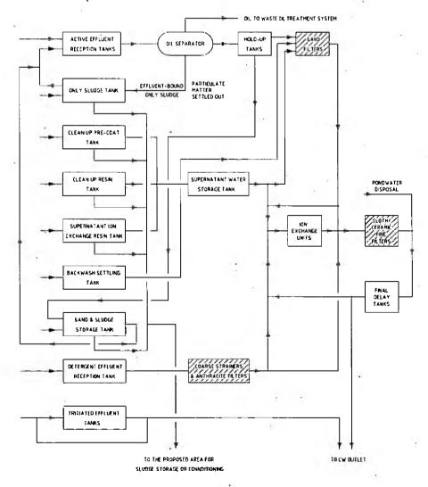
the pond water needs to be discharged (a very rare occurrence), it is bled off from the ponds via the PWTP ion exchange beds for initial clean-up prior to being passed to the AETP for final treatment and discharge.
