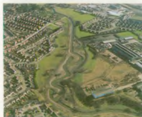
Restoring lost channel features - reinstated meanders on the River Skerne, Darlington
