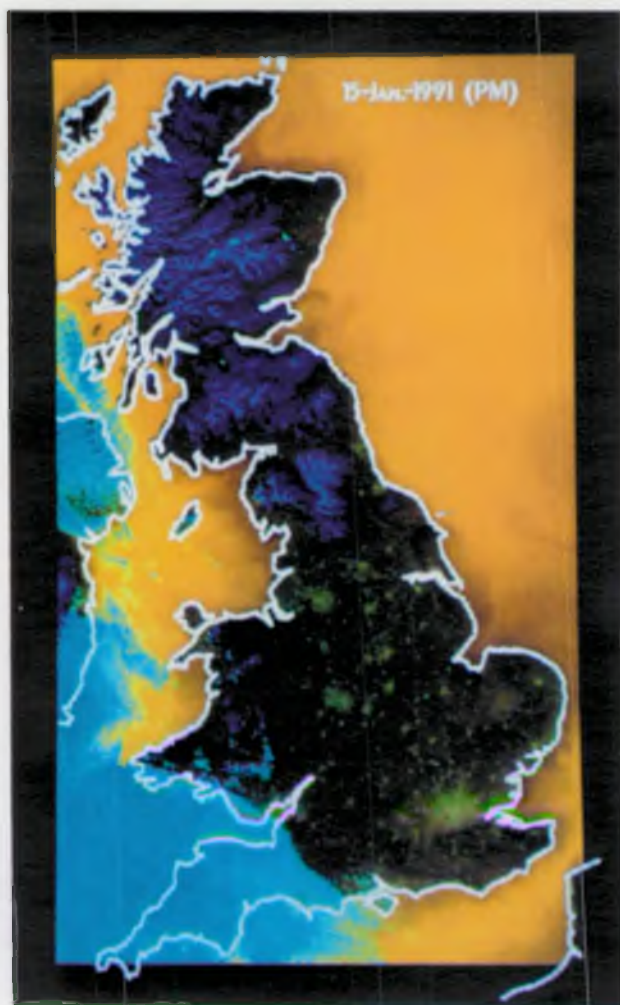
Plate 3.4 Colour composite of calibrated NOAA-11 AVHRR band-1 (blue), band-3 (green) and band-4 (red) of the UK, 15 January 1991.
