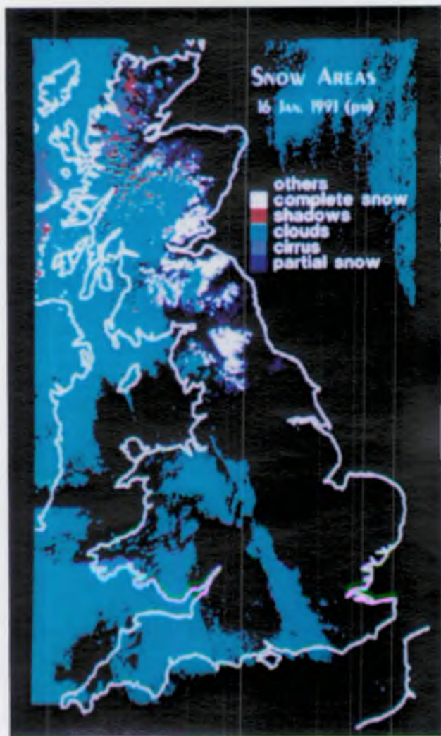
Plate 3.2 Snow area mapping for 16 January 1991 following the procedures in Figure 3.1 with identification of shadows, cirrus and partial snow and complete snow.
