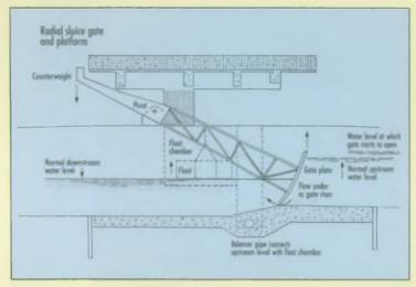
The radial gate opens automatically as levels rise upstream. A pipe connects to float chambers either side of the gate. As the levels rise, so large hollow metal boxes connected to the gate float up overcoming the counterweight. This raises the gate plate, allowing more water to flow through
