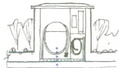
50MM DIA FLEXIBLE SUCTION HOSE, COIN OPERATED PUMP SWITCH AND 12MM DIA FLUSHING HOSE HOUSED IN BRICK SHELTER WITH PRECAST CONCRETE ROOF. SET ON CONCRETE BASE WITH BRICK TRIM
