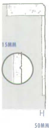
① SCRIBED GUNITE FACING 'BLOCKWORK EFFECT'
