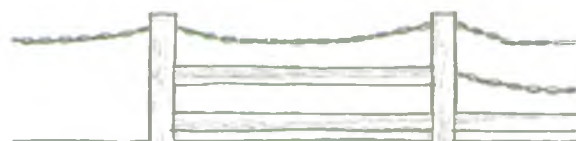
POST & MORTICED RAILS IN COMBINATION WITH STRUNG CHAINS: CREATES A MORE LIGHT WEIGHT BARRIER NOTE: VARIOUS ARRANGEMENTS OF RAILS & CHAINS
