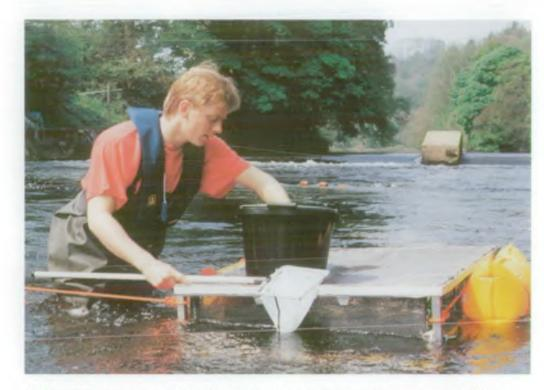
Wild smolt trapping at Manley Hall using a floating fyke net and holding box suspended below the right bank weir
