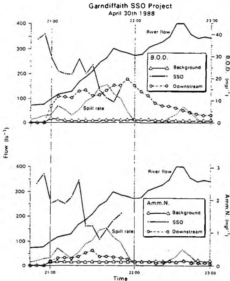
Fig. 2. Typical SSO spill impacts
