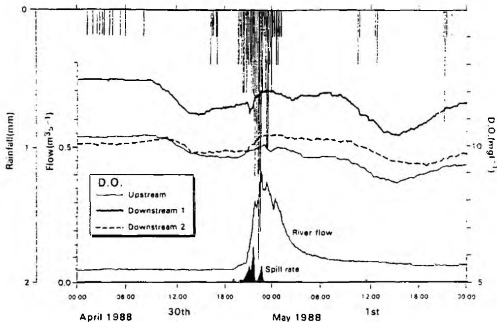
Fig. 1. Typical SSO response timing and D.O. impact
