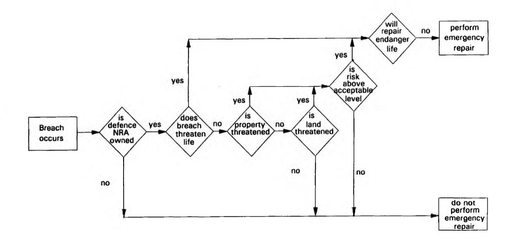
Figure 6.3 Flowchart Outlining Decision to Perform Emergency Repair or Not
