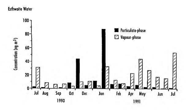
Figure 4.2 Concentrations of polycyclic aromatic hydrocarbons measured in high volume air samples from Castleshaw and Esthwaite Water, July 1990 - July 1991
