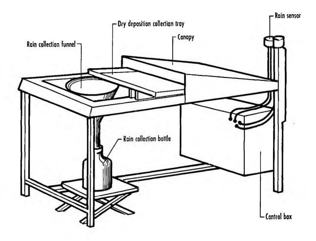
Figure 3.1 Diagram of automatic wet and dry deposition collector
