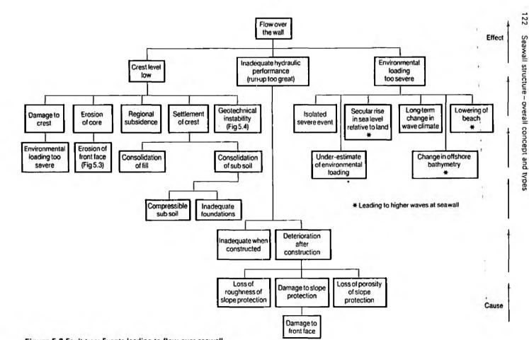
Seawall structure overall concept and types
