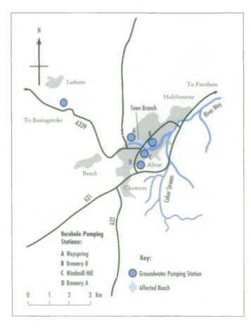
river flow. The 5 megalitres a day output from the two stations will be made up from a new borehole to be sunk into the Chalk and Upper Greensand aquifers south-west of Alton, away from the river.
