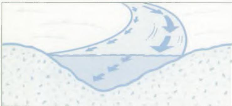
The **velocity** of water in a river usually decreases with depth and increases toward the outside of bends.
