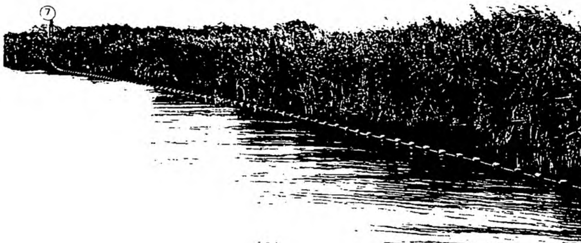
5.1 REED GROWTH THROUGH ASPHALT MATTING LAID ON GRADED BANK
