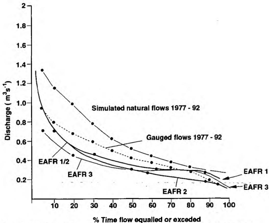
Figure 2b flow duration curves for three EAFR scenarios defined in the text in comparison to the gauged air simulated return data
