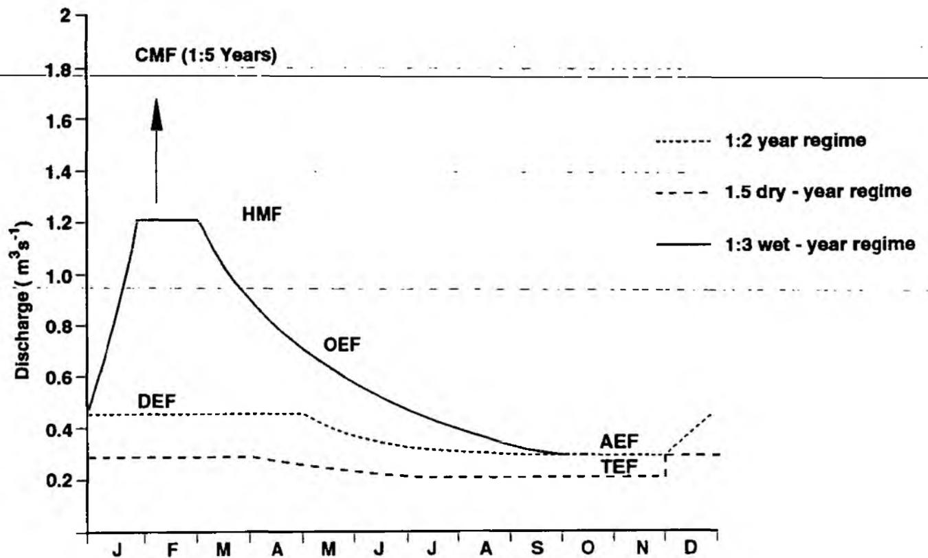
Figure 2a Flow Hydrographs used to construct the EAFR for the River Babingley
