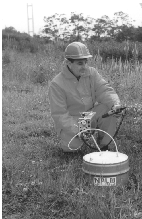
Figure 5.1: Cylindrical Flux Chamber (Developed for Monitoring Methane Emissions from the Surface of Landfill Sites)
