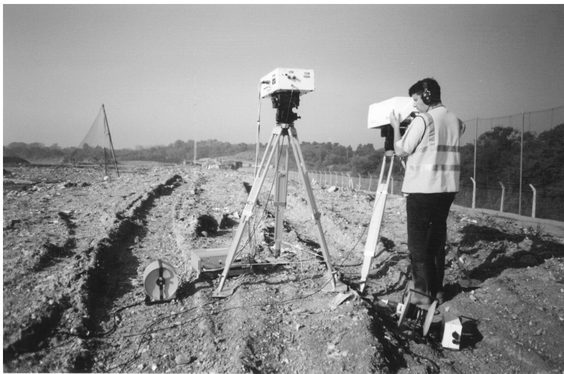
Figure 5.4: Optical Integrated-Path Monitoring Using a HAWK Infrared Monitor Along One Side of a Landfill Site
