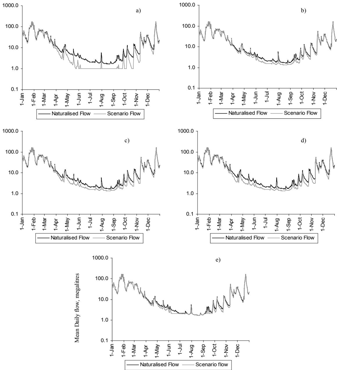
**Figure 7. Hydrographs of flow regime in 1995 with abstraction rules, a) Rule I, b) Rule II, c) Rule III, d) Rule IV and e) Rule V.**
