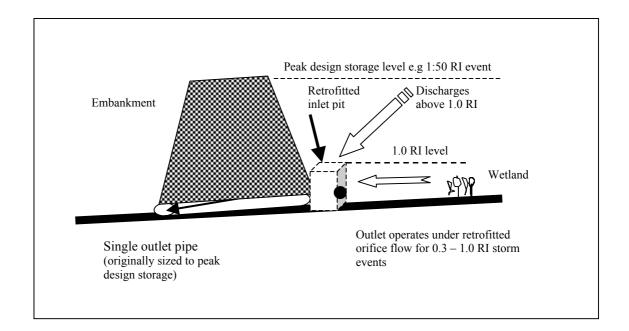
Figure 2.8. Retrofitting a Dual Outlet to Flood Storage Pond
