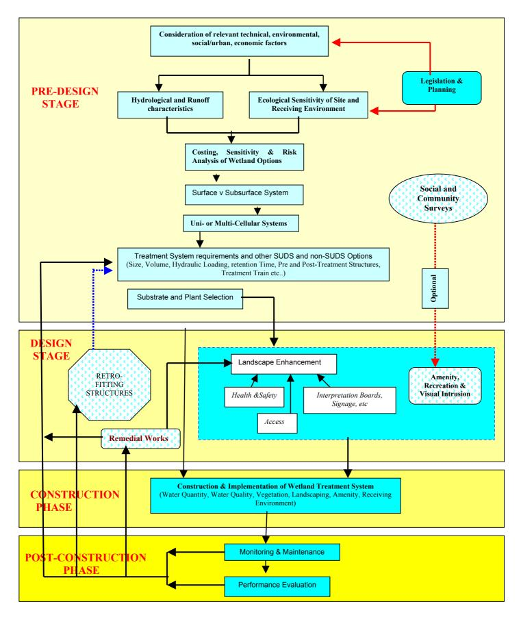
Figure 7.2 Process Diagram for the Design of Constructed Wetlands
