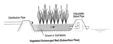
Figure 1.2b. A SSF Constructed Wetland Illustrative Cross-section (After: Kadlec and Knight, 1996)
