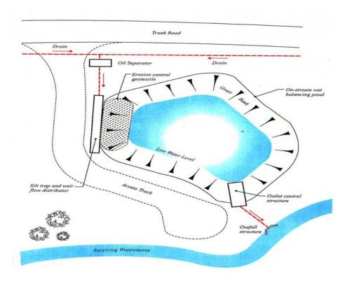
Figure 2.5 Original On-Stream Wet Retention Balancing Pond Before Retrofitting
