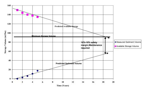
Figure 4.1 Predicting Sediment Removal Maintenance Requirement Time
