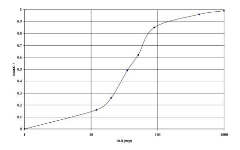
Figure C1. Bacterial Removal Efficiency and Hydraulic Loading Rate
