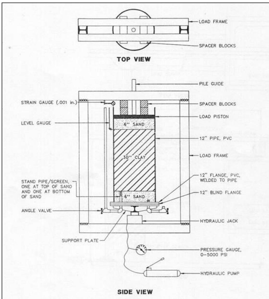
Figure 2.2. Test configuration used by Hayman et al. (1993) (after Hayman et al. 1993)
