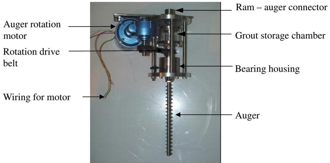
**Figure 3.3. Model CFA piling equipment**
