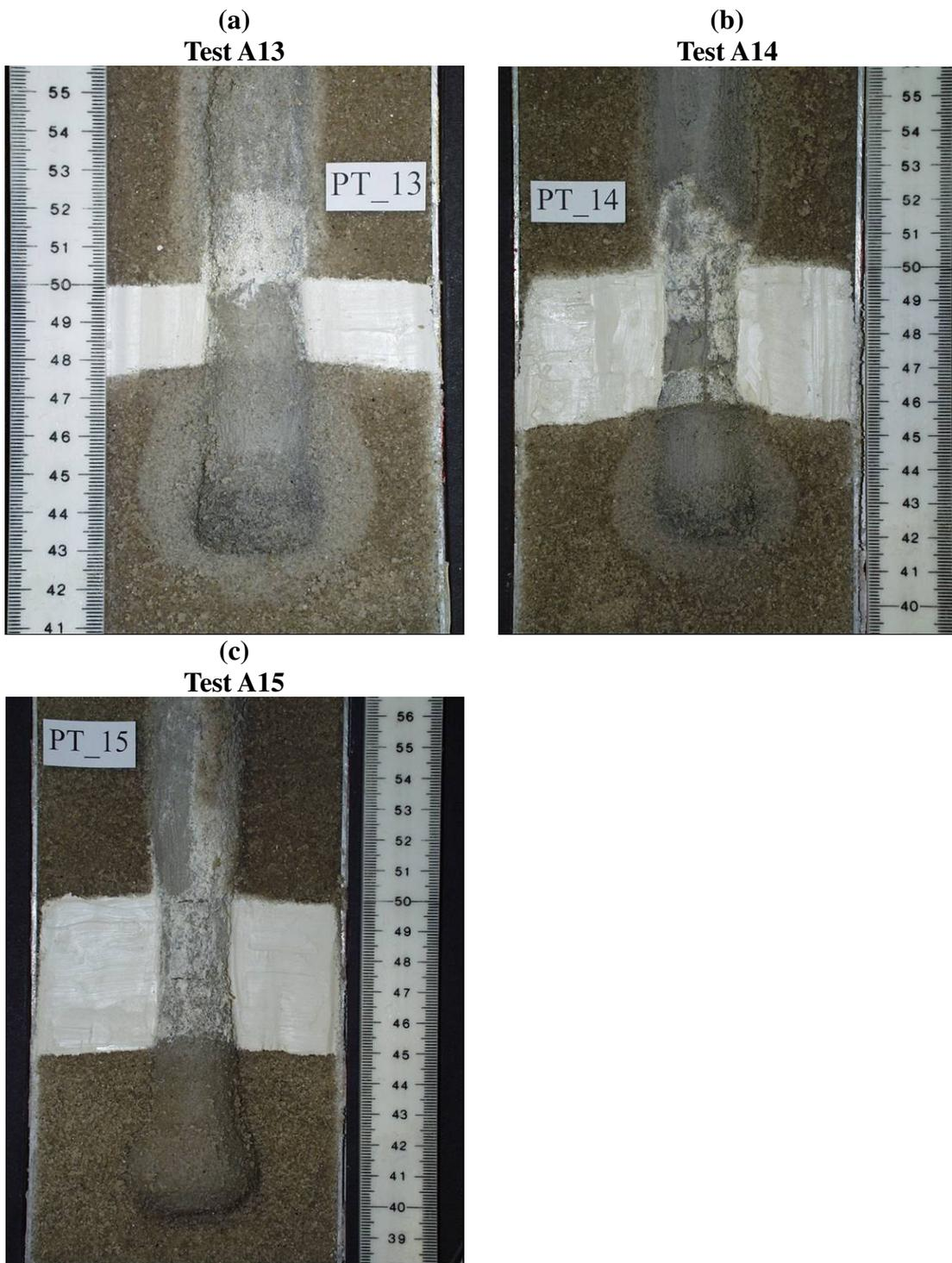
Figure 4.3. Photographs of dissected axisymmetric models: CFA piles
