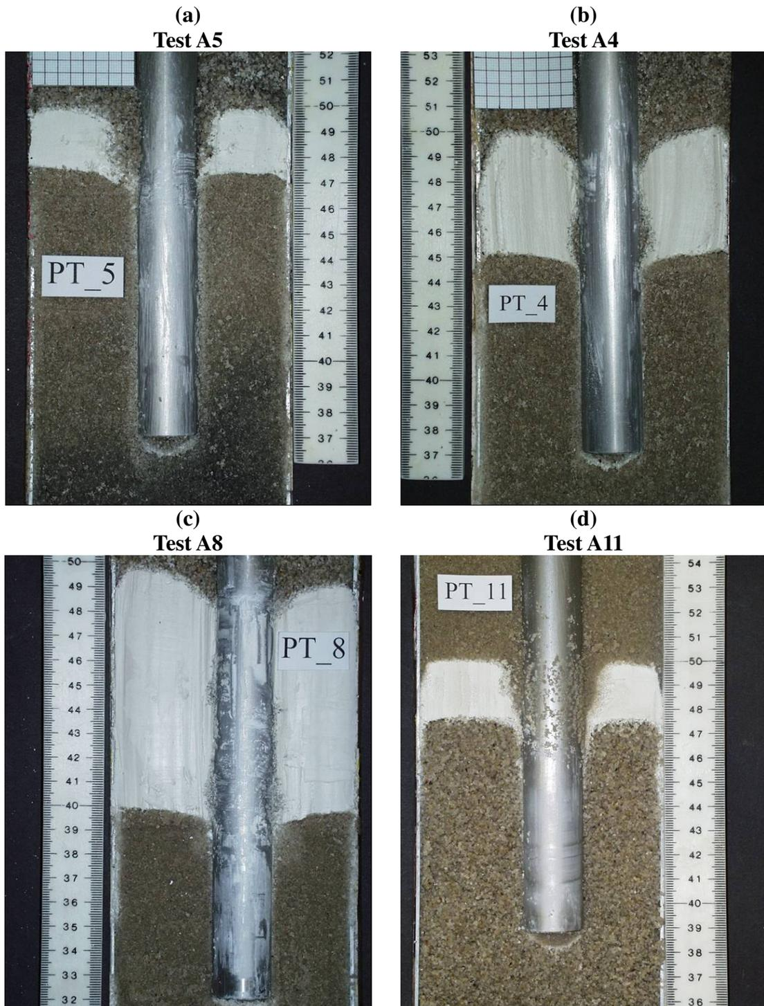
Figure 4.1. Photographs of dissected axisymmetric models: cylindrical piles
