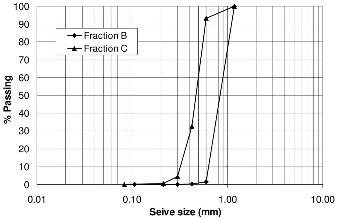
**Figure 4.14. Particle size distributions of sands used in the models**
