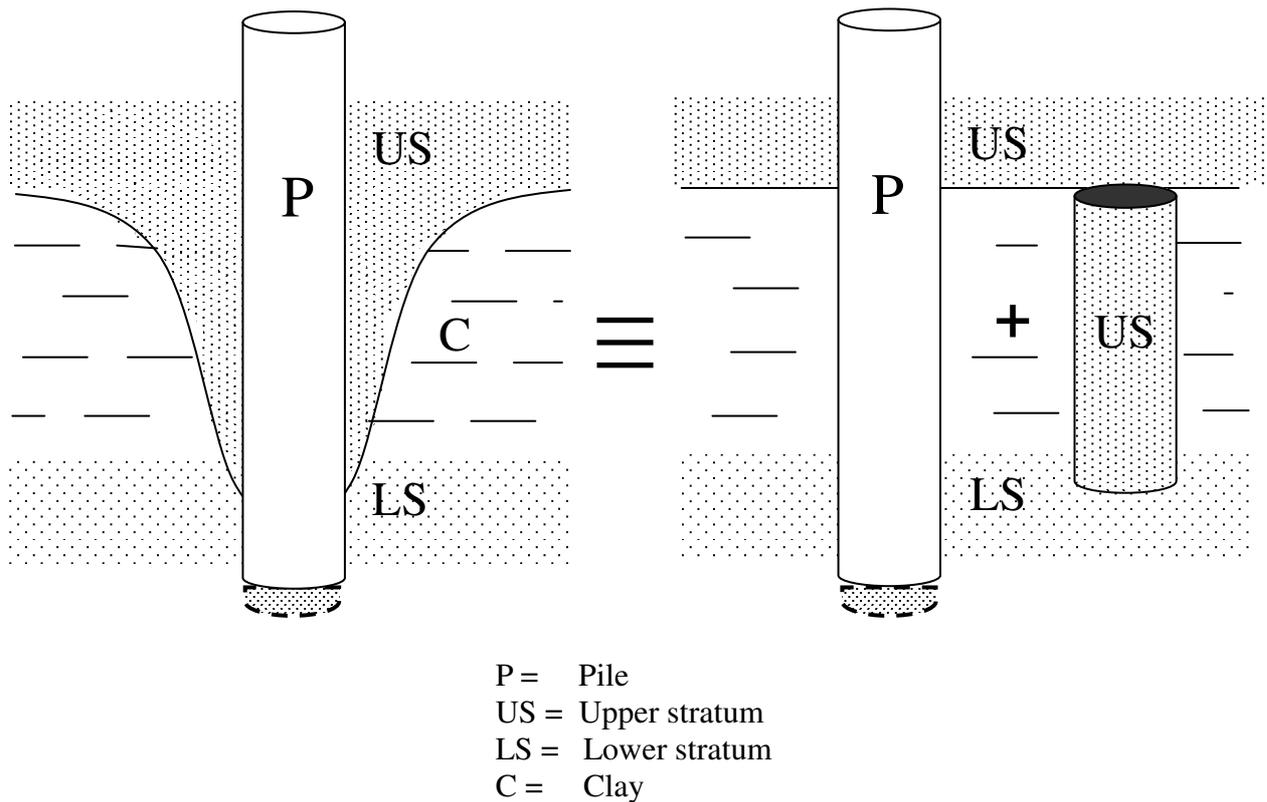
\* Note: a similar concept applies where the upper stratum is carried down within the flanges of an H-section pile.
