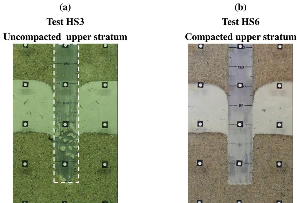
**Figure 4.5. Photographs of half-section models: H-section piles**
