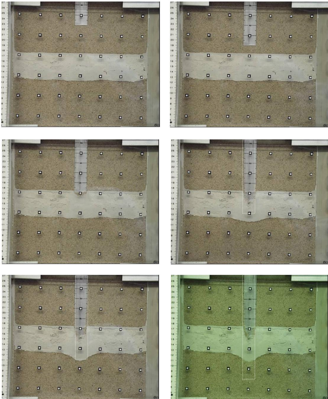
**Figure 4.10. Photographs of penetration stages in a half-section model: cylindrical pile through a stiff clay layer**
