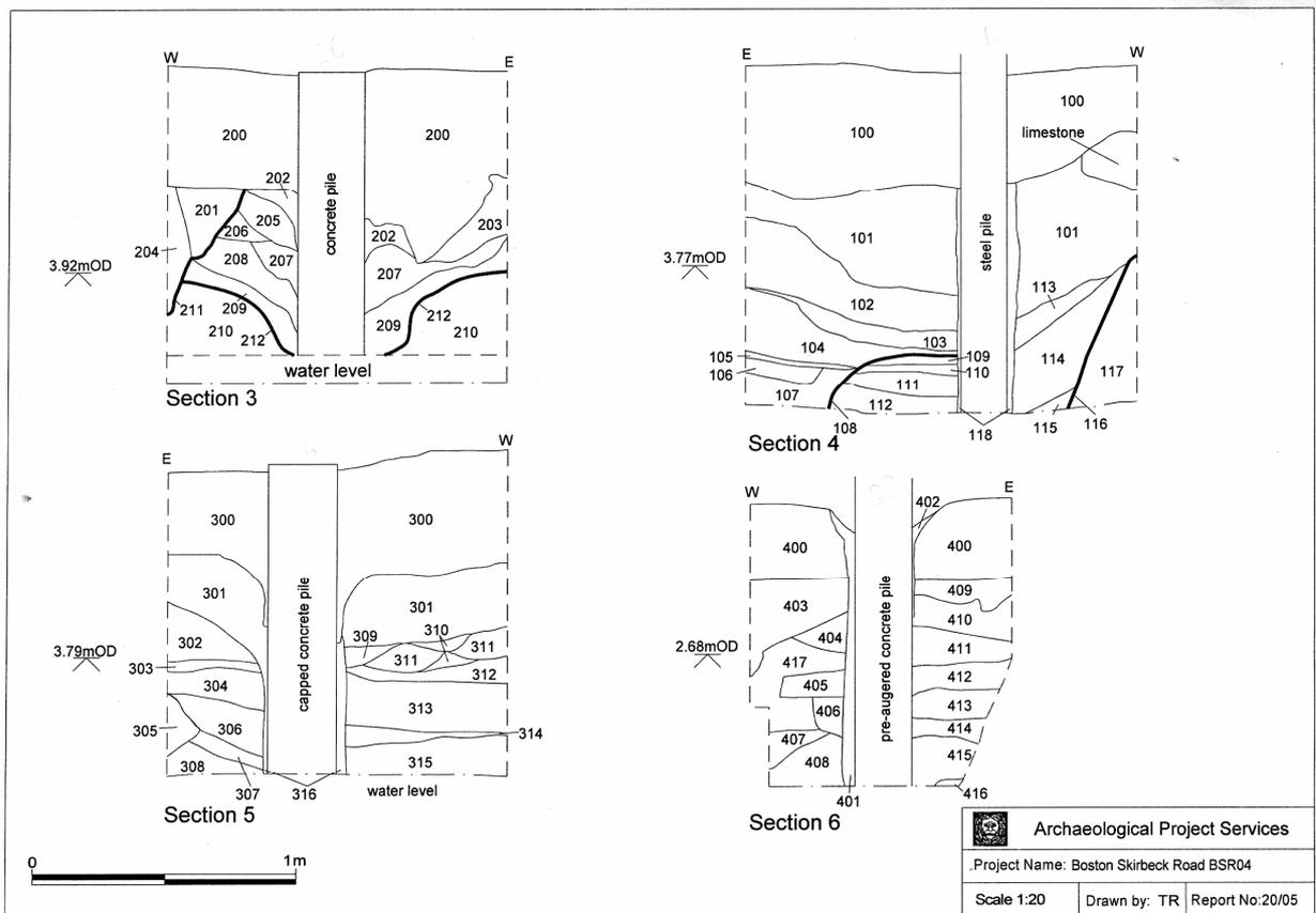
Figure 5: Pile Sections (No's 3 - 6)
