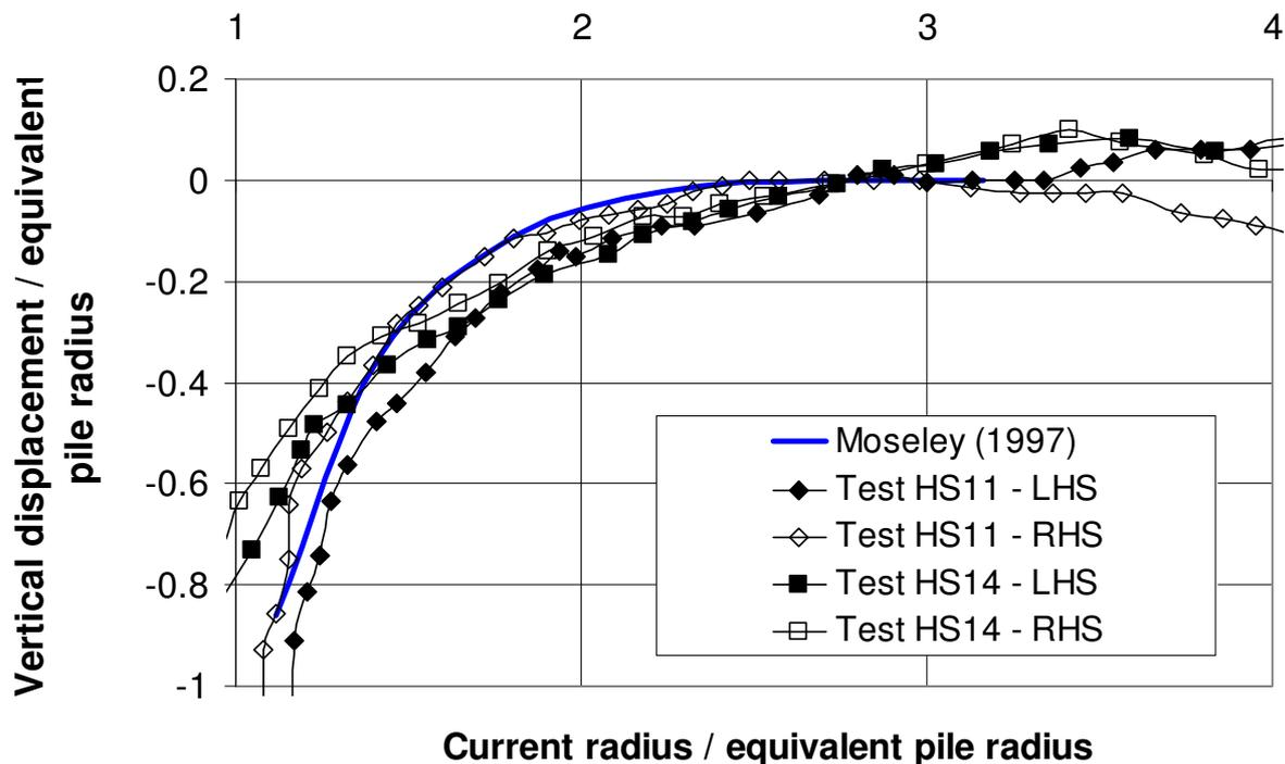
**Figure 4.20. Comparison of present and previous results for vertical displacement adjacent to driven piles in clay**
