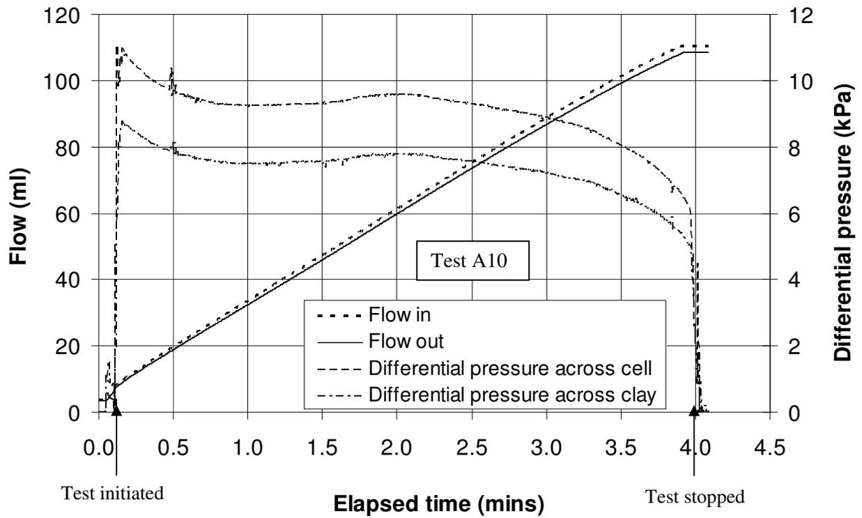
Figure 4.17. Example of header tank test result after model pile construction
