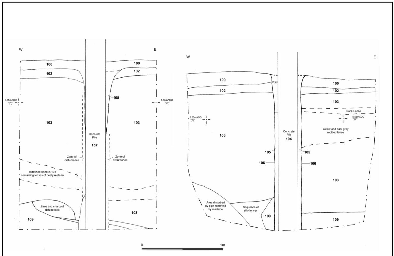
**Figure 5.5. Sections showing disturbance caused by driven and pre-augered driven concrete piles at Lincoln. Numbered zones (except 104 and 107) represent various soils.**
