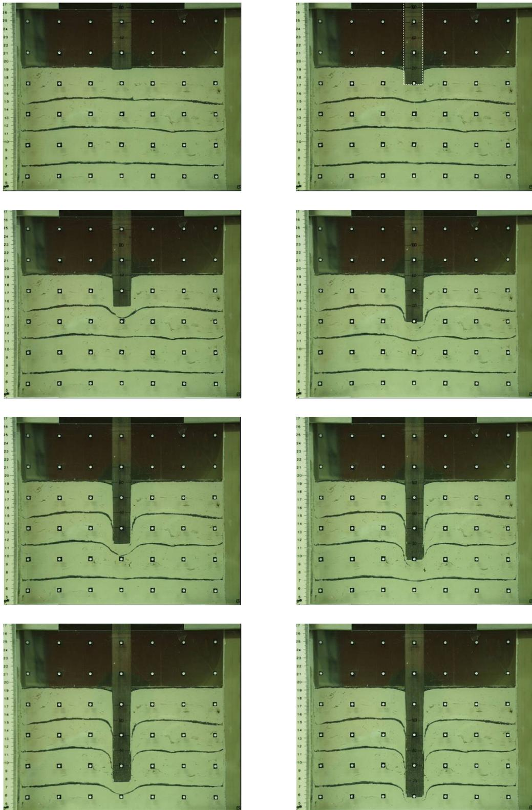
**Figure 4.11. Photographs of penetration stages in a half-section model: square pile through homogeneous soil**
