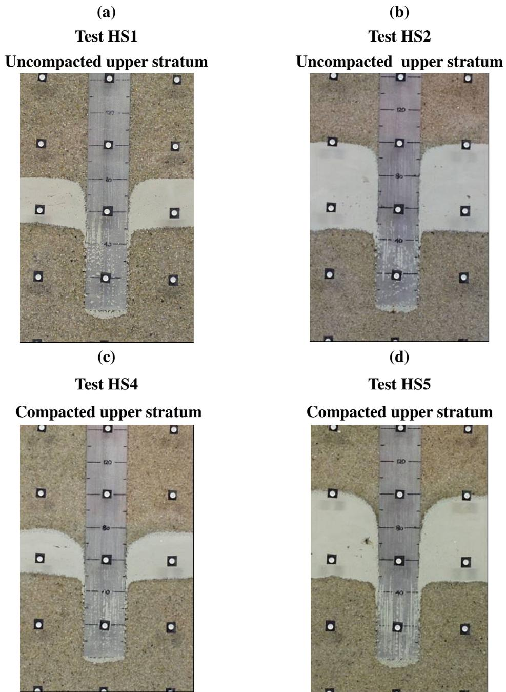
Figure 4.4. Photographs of half-section models: cylindrical piles
