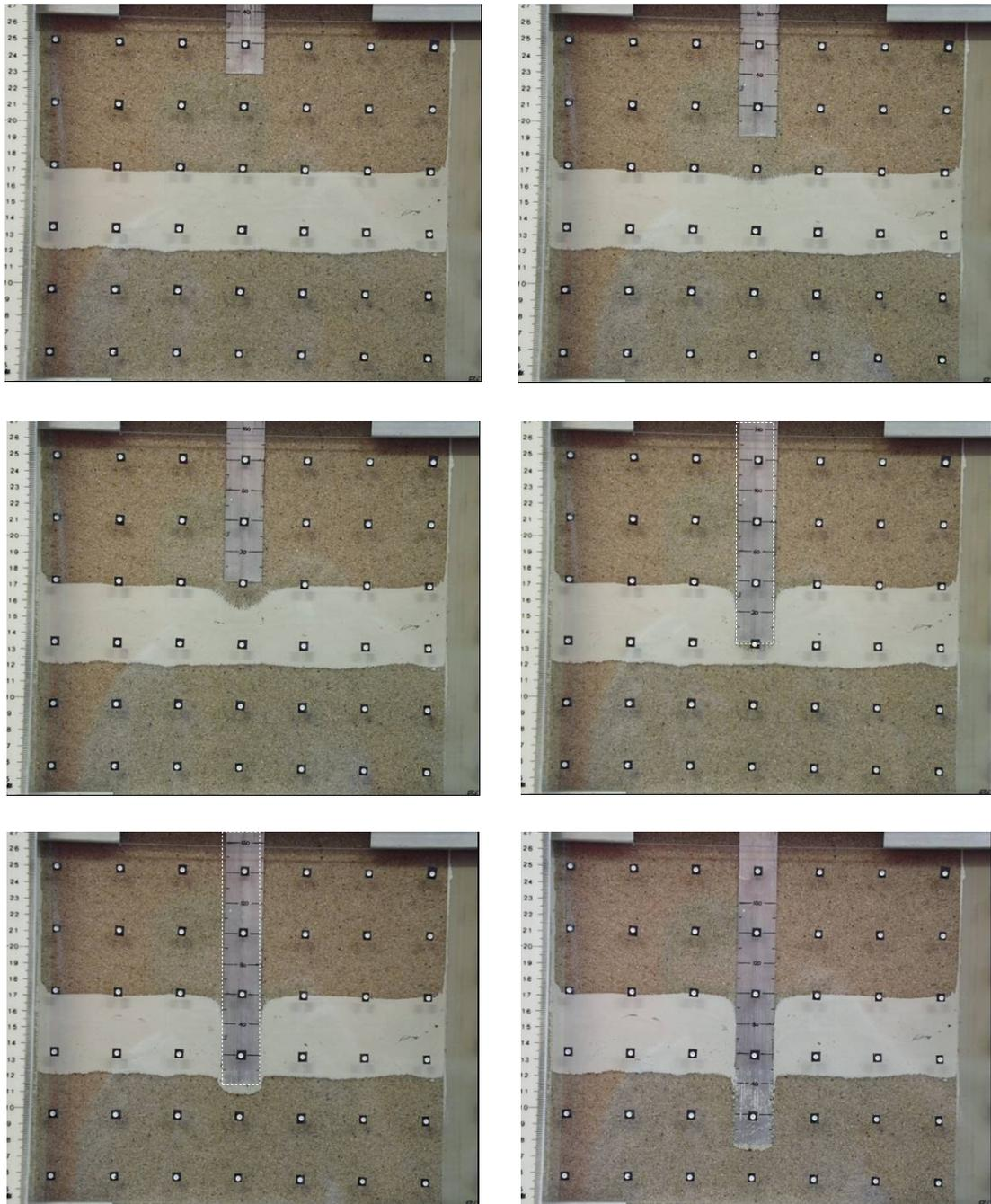
**Figure 4.9. Photographs of penetration stages in a half-section model: cylindrical pile through a soft clay layer**
