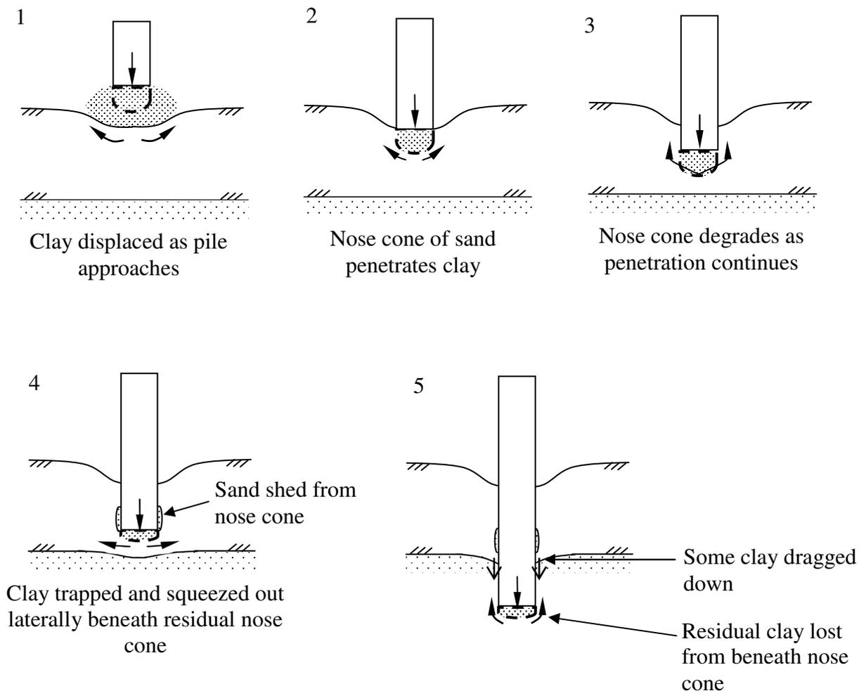
**Figure 4.12. Schematic diagram of penetration stages in layered soil**
