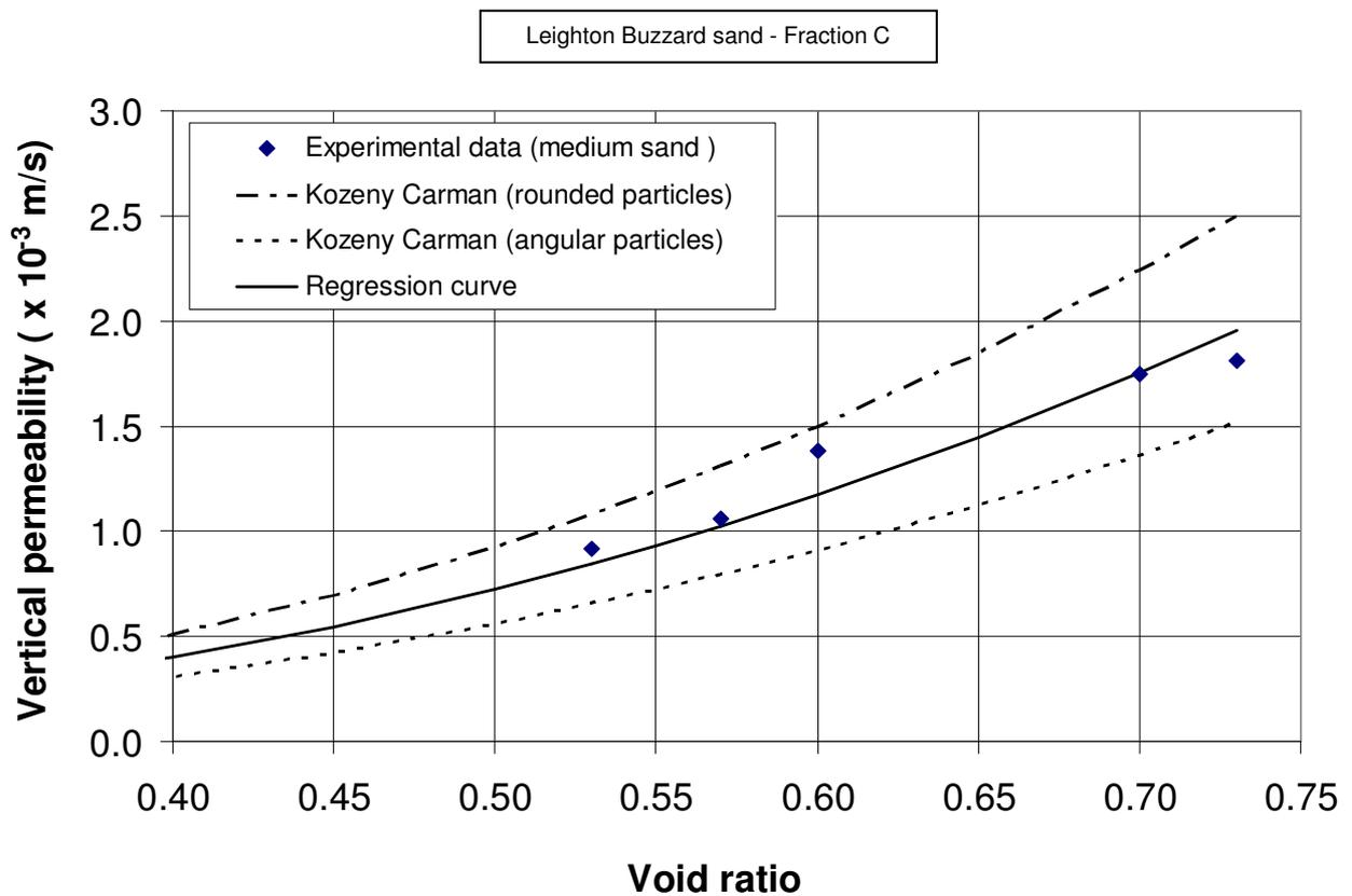
Figure 4.15. Permeability variation with void ratio for sands used in the models
