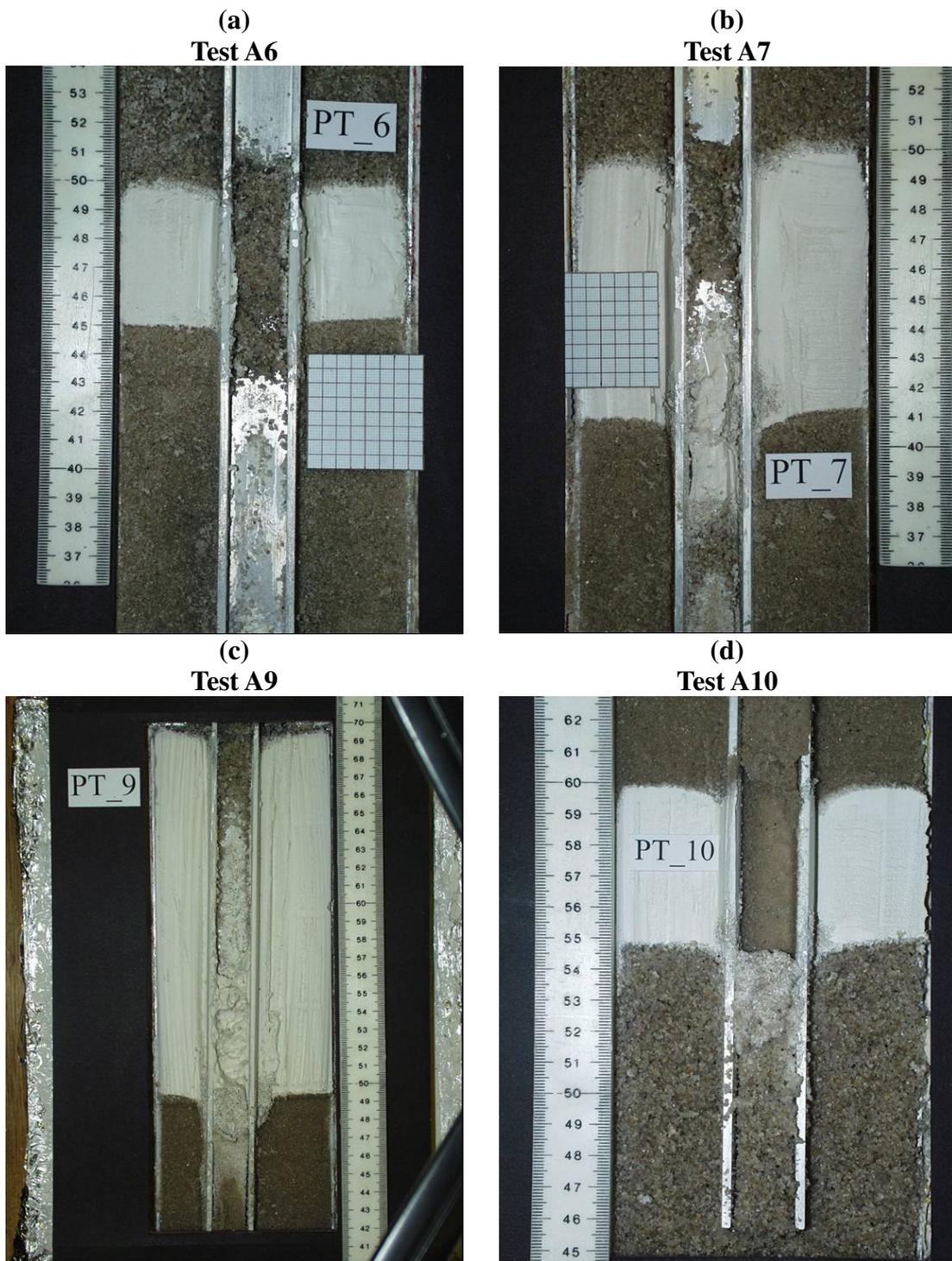
Figure 4.2. Photographs of dissected axisymmetric models: H-section piles
