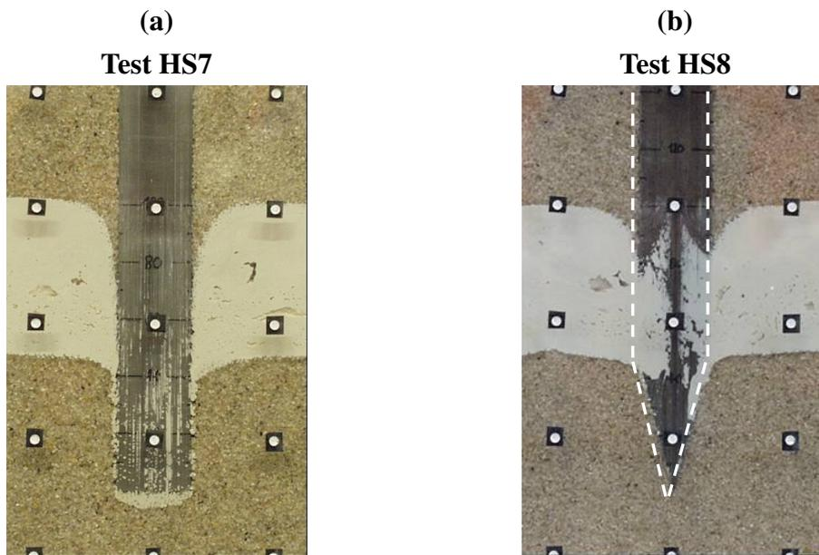
Figure 4.6. Photographs of half-section models: square piles
