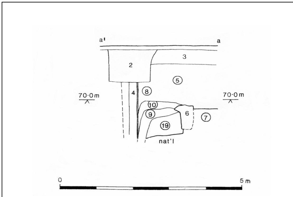
**Figure 5.1. Section showing disturbance due to a pile at Barclaycard Marefair Northampton (reproduced by permission of the Historical Environment Team, copyright Northamptonshire County Council). Zone 2 represents the pile cap, zone 4 represents the pile and the remaining zones represent various soils.**
