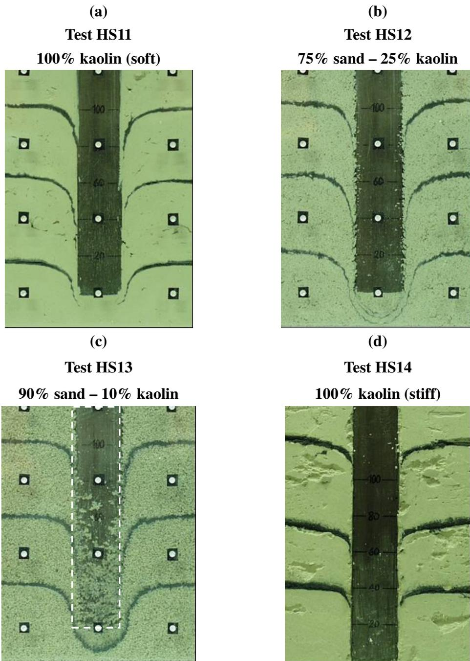
Figure 4.8. Photographs of half-section models: square piles in homogeneous soil
