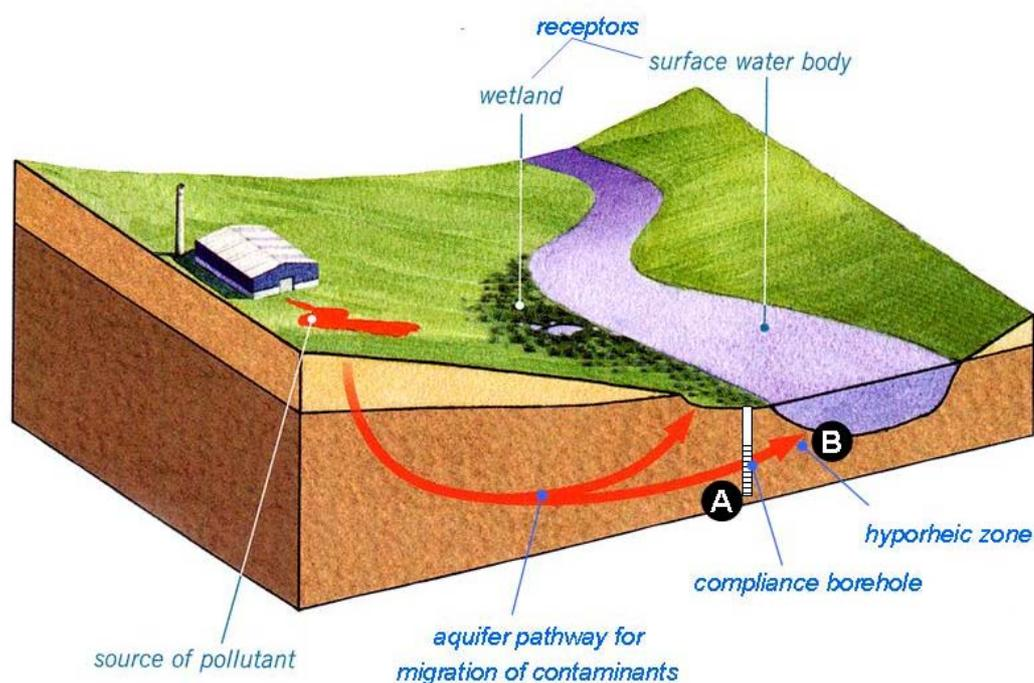
**Figure 2.4 Typical contaminated-site assessment using the *source–pathway–receptor* framework. Use of a compliance-monitoring borehole adjacent to the stream (A) excludes any potential attenuation capacity within the hyporheic zone (B). (Based on Environment Agency 2002.)**
