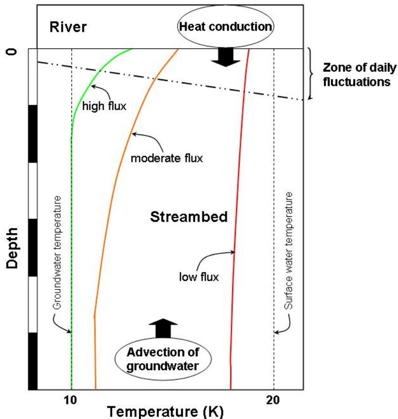
**Figure 3.3** Illustrative temperature versus depth profiles through the hyporheic zone for systems with high, moderate and low upwards groundwater flux (based on Conant 2004).
