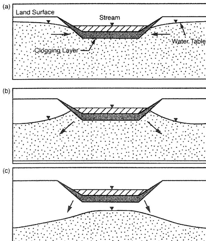
**Figure 3.4 River–aquifer relationships for (a) gaining stream, (b) connected losing stream and (c) disconnected losing stream (after Sophocleous 2002, © Springer-Verlag 2002).**
