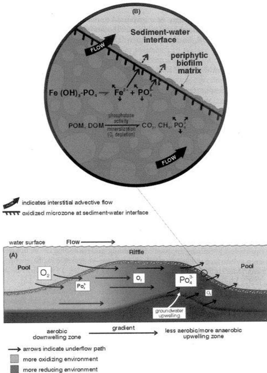
Figure 4.2 Conceptual model of hyporheic flow paths through an idealised riffle, showing changes of oxygen and phosphate concentrations in response to the aerobicity of interstitial waters. Relative concentration is indicated by the size of white box (based on Hendricks and White 2000, © Academic Press, Inc. 2000).
