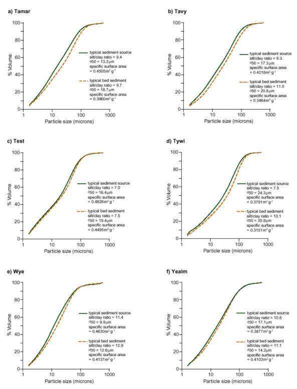
Figure 3.5: Comparison of the typical absolute particle size composition of source material and interstitial sediment samples
