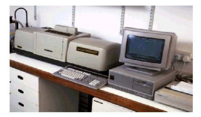
Plate 3.1: The laser diffraction granulometer.
