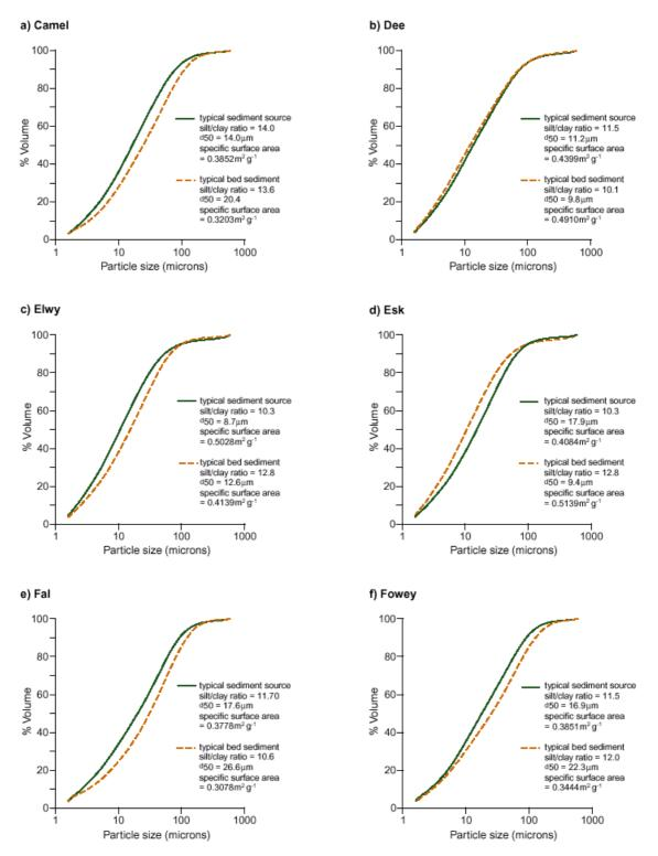
Figure 3.3: Comparison of the typical absolute particle size composition of source material and interstitial sediment samples
