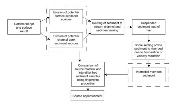
Figure 3.1: The basis of employing the fingerprinting approach to establish the provenance of interstitial fine sediment recovered from spawning gravels
