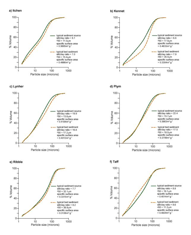
Figure 3.4: Comparison of the typical absolute particle size composition of source material and interstitial sediment samples
