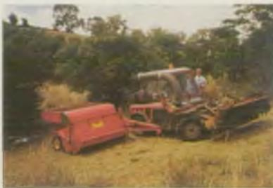
Weed harvester carrying out weed control and cutting. The cut weed is collected and stored on board until being off loaded onto the river bank at convenient locations.
