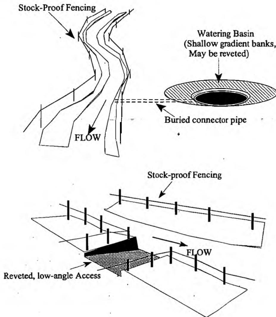
**Figure 5: Example of an On-line Watering Structure.**
