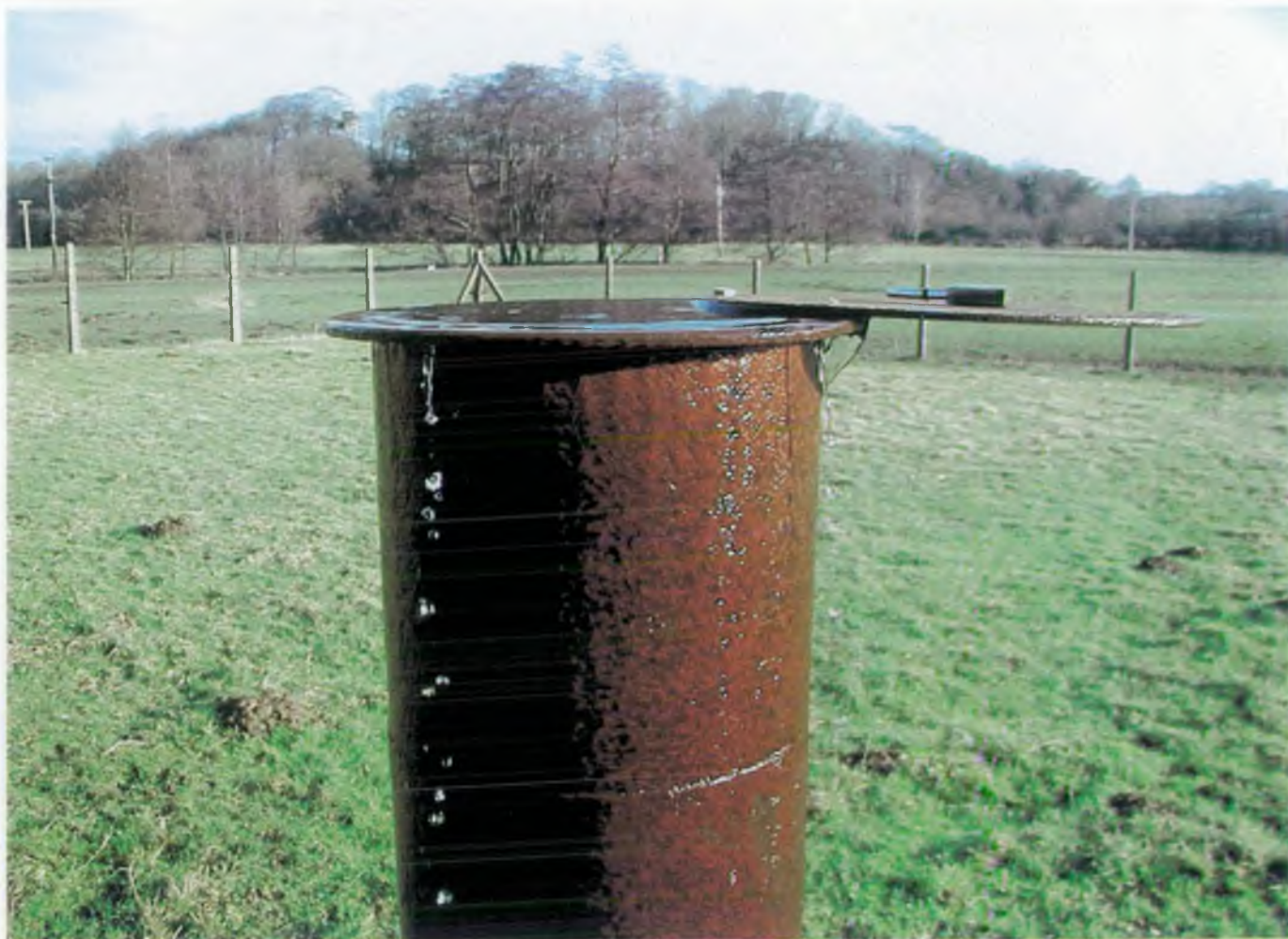
Figure 45: Overflowing observation borehole, TL32/7, TL 386 247, Braughing, River Rib.
