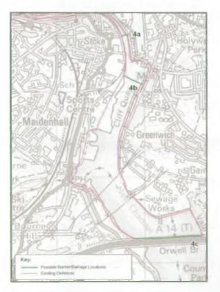
Figure 5 Indicative locations for barrage/barrier
